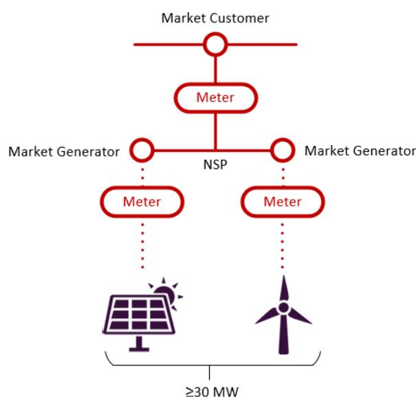
This registration would involve two semi-scheduled generating units; one wind and one solar (each aggregated under NER 2.2.7). The two systems are connected into the private network and operate independently of each other with individual registration, conformance cap, GPS (which need to consider each other in the modelling), dispatch, SCADA and ECM.
