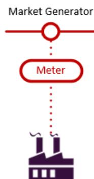
A synchronous generating system, for example, open cycle or combined cycle gas turbines, hydro or coal-fired power stations, would be classified as scheduled and be connected to the NEM via a single connection point with its own metering installation represented by a NMI.
