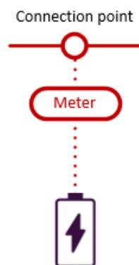
A battery would be classified as a scheduled generating unit, and also a scheduled load (requiring Market Customer registration) if it intends to charge from the grid. It would be connected to the NEM via a single connection point with its own metering installation represented by a NMI.
