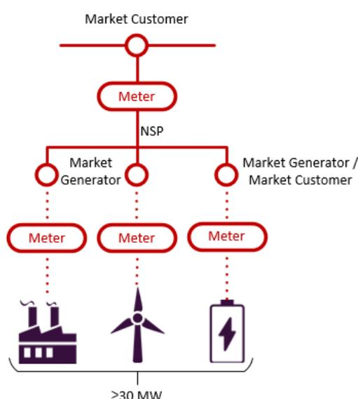
This scenario includes a semi-scheduled generating unit and two scheduled generating units: one wind farm, one gas fired turbine, and one battery that charges from the grid. The three systems are connected into a private network and operate independently of each other with individual registration, conformance cap for wind farm, GPS (which need to consider each other in the modelling), dispatch, SCADA and ECM for the wind farm.
