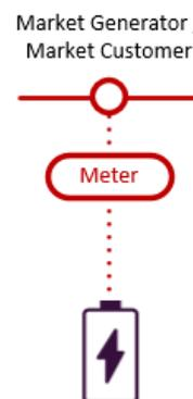
A battery <5 MW is typically exempt from registration but can be classified as a non-scheduled generating unit. This is the case if a <5 MW battery is part of a hybrid system which is  $\geq 5$  MW. Other generating technologies (including wind, solar and synchronous) are usually classified as non-scheduled if the system is <30 MW.
