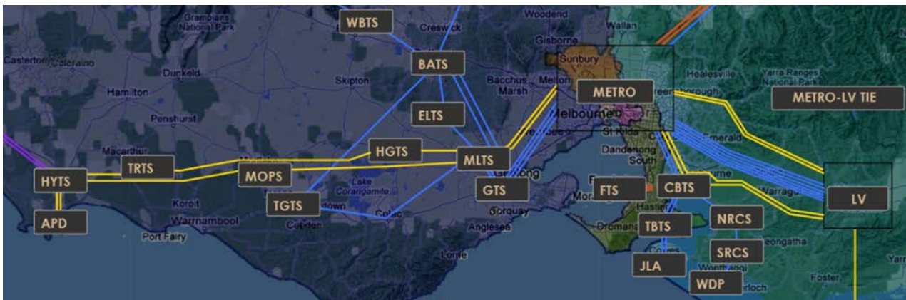
Figure 2 - 500 kV Transmission Backbone
