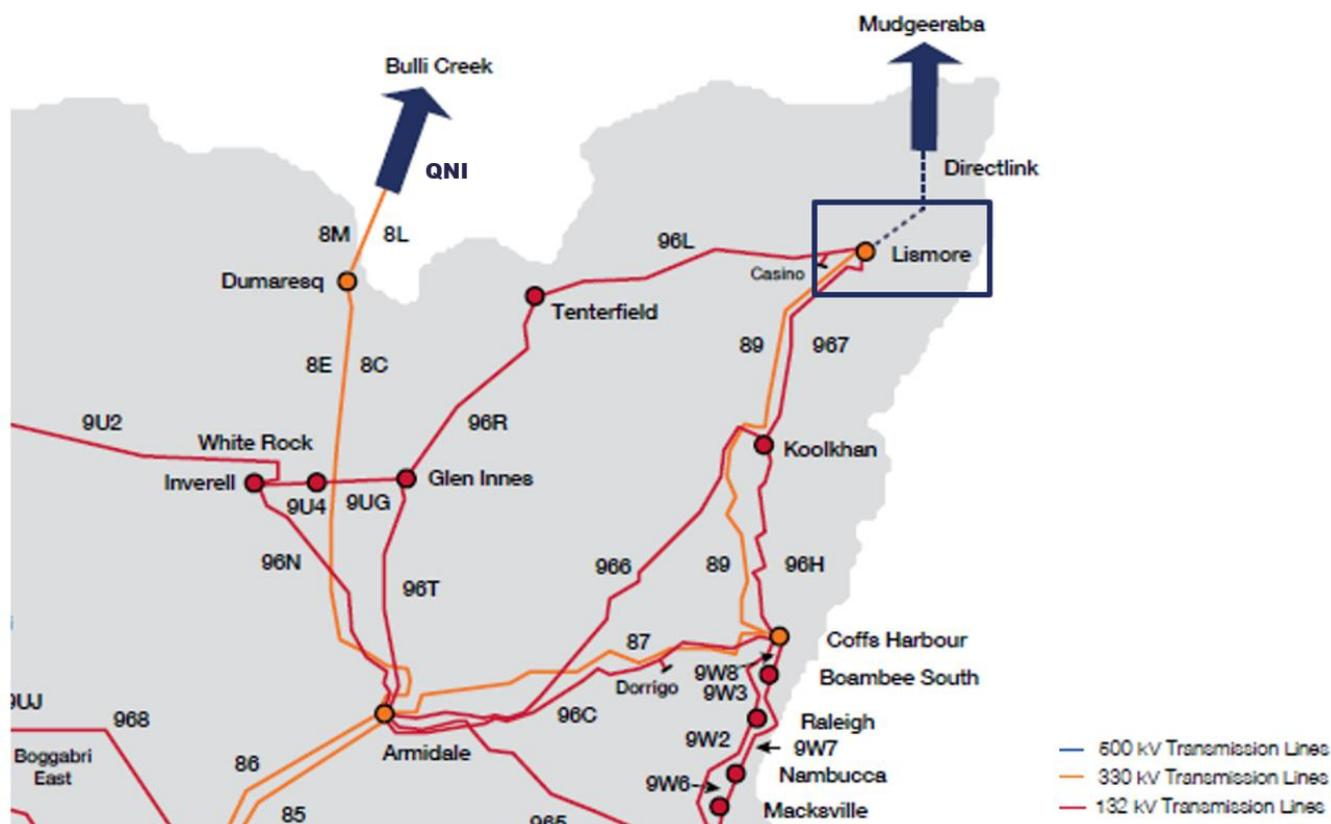
Converging to Lismore substation, Lines 87 and 89 connect Armidale to Lismore via Coffs Harbour and together span approximately 300 km. Two additional 132 kV transmission lines also terminate at Lismore: Line 967 which spans approximately 90 km from Koolkhan to Lismore and Line 96L which spans approximately 122 km from Tenterfield to Lismore. These transmission lines play central roles in supplying this part of the network.
