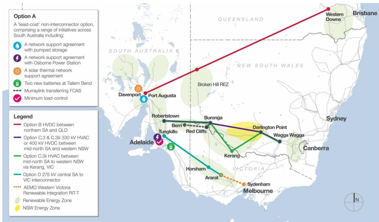
While a stylised straight-line representation of interconnector routes has been included in the figure above for simplicity, detailed desk-top assessments have been undertaken to identify notional routes for each option. Indicative estimated costs of land and easement acquisition have been factored into the cost estimates for the various interconnector options based on this analysis.
