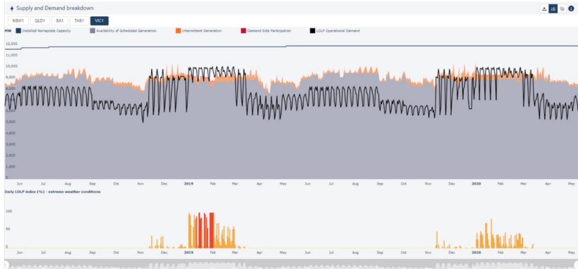
Figure 14 Supply demand breakdown and maintenance period overview from LOLP run (user to select region and year)
