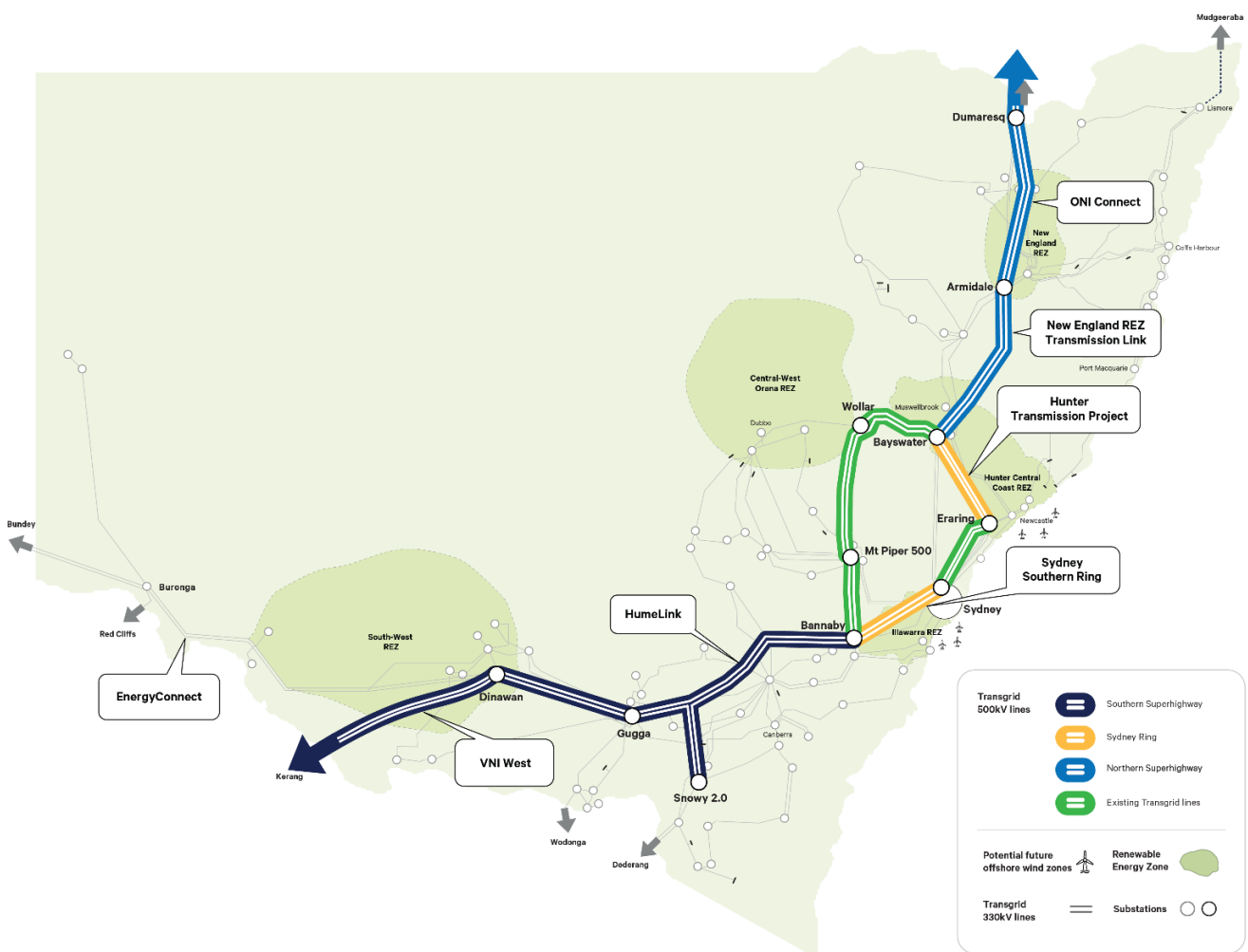
Figure 1 NSW Energy Superhighway
