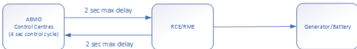
Maximum end to end timing for control commands from AEMO control centre to RCE/RME
