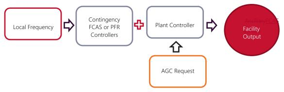
Hence, where relevant, Contingency FCAS or PFR controllers must detect Local Frequency and calculate an appropriate response. The <u>FCASAncillary Service</u> Facility's Plant Controller should take the sum of the response calculated by the Contingency FCAS or PFR controllers and response requested by the AGC control signal to determine the required output from the <u>FCASAncillary Service</u> Facility.
