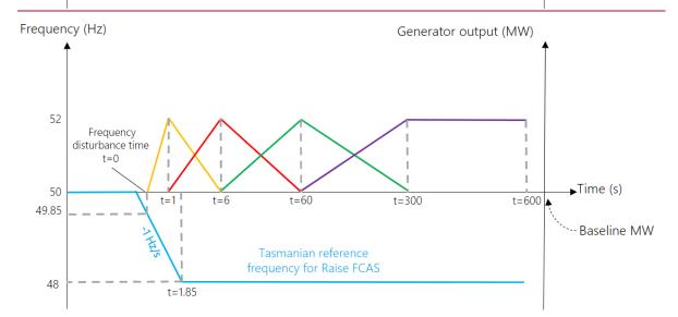
Figure 9 shows an example of how a simple Variable Controller that supplies a droop-based response to a Frequency Disturbance can deliver across the Contingency FCAS timeframes by an FCAS Provider also registered in the Very Fast FCAS markets.
