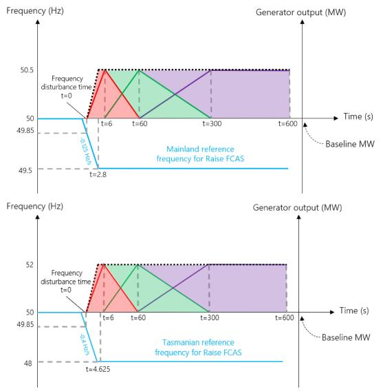
Figure 8 shows a visual representation of the measurements applied to verify that at least the minimum required Contingency FCAS has been delivered in each timeframe by an FCAS Provider also registered in the Very Fast FCAS markets.
