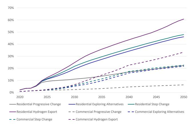
Figure 5-7 Projected share of solar-PV systems with a battery by customer type
