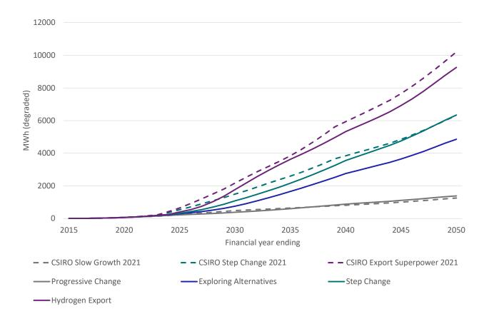
Figure 5-6 Projected capacity of small-scale batteries in the SWIS
