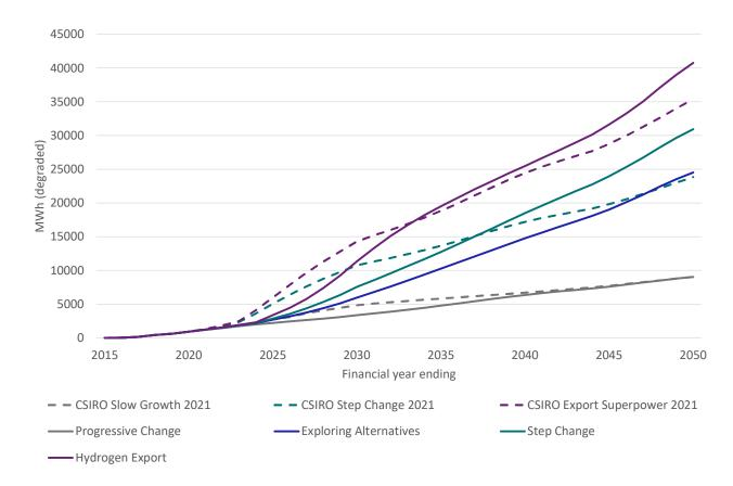
Figure 5-5 Projected capacity of small-scale batteries in the NEM
