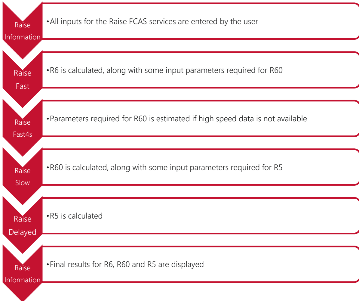
Figure 3 FCAS VT calculation process - Raise
