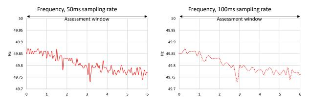
Figure 7. Example of local frequency measurement for the six-second assessment window, with 50ms (left) and 100ms (right) sampling rates, for event 2
