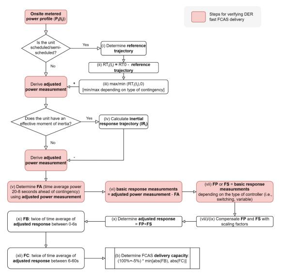
Figure 1. Fast FCAS performance verification methodology (redrafted from [1])
