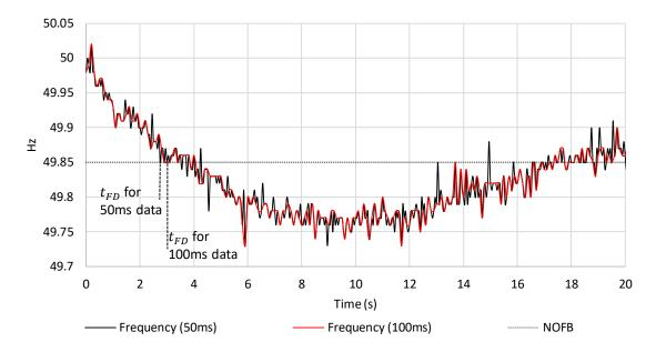
Figure 6. Example of local frequency measurement and identification of the frequency disturbance time of an NMI with 50ms and 100ms sampling rates, for event 2
