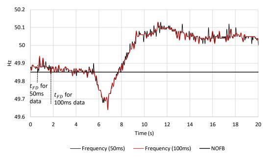
Figure 4. Example of local frequency measurement and identification of the frequency disturbance time of an NMI with 50ms and 100ms sampling rates, for event 1
