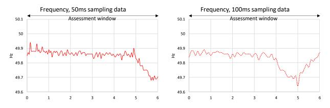
Figure 5. Example of local frequency measurement for the six-second assessment window, with 50ms (left) and 100ms (right) sampling rates, for event 1
