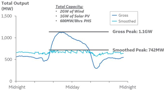
Potential to replace a 1.1GW line at ~60% utilisation with a 742MW one at ~90% utilisation
