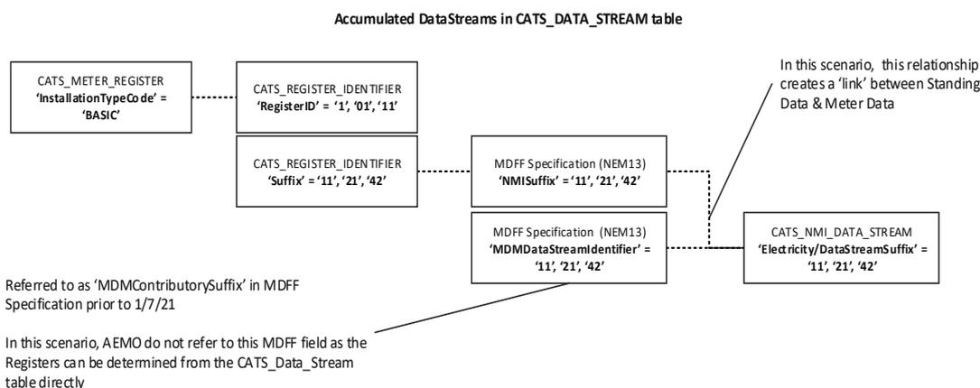
Example of an Interval Meter ‘Suffix’ – Net DataStreams
