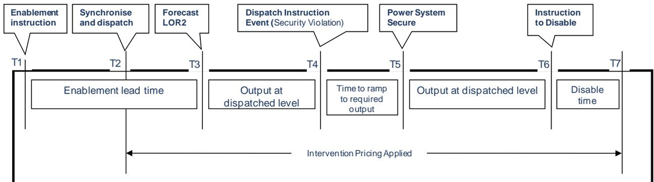
Enablement means preparing the *reserve equipment* to be *dispatched*. For example, Figure 1 demonstrates a fast response generator that does not need to be synchronised at the forecast LOR2 time (T2) to provide the reserve capacity. Note: a slow response generator may require *synchronising* and *loading* to its *minimum operating level* or some nominated level at the start of the LOR2 period (as shown in Figure 2), so that it can provide the reserve capacity within the timeframe required.
