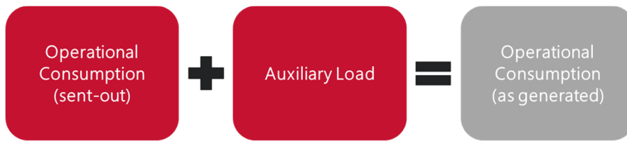
Figure 15 Figure 16 Converting from operational consumption (sent-out) to operational consumption (as generated)
