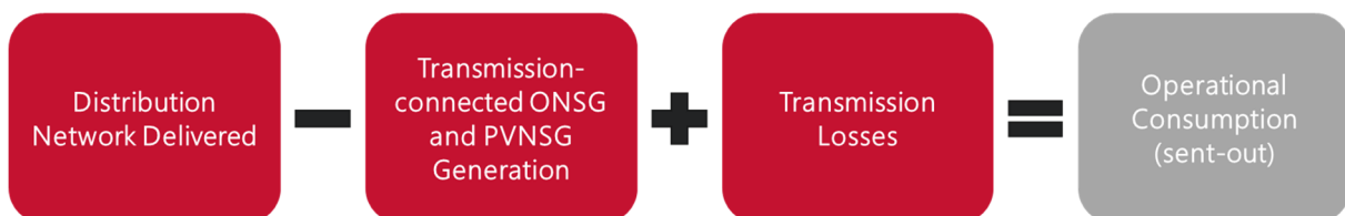
Figure 14 Figure 15 Operational consumption (sent-out)
