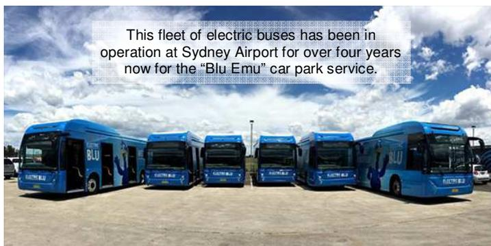
These buses use batteries of around 330kWh capacity and consume around 80kW per hour under normal driving conditions. Buses typically operate for long hours during the day, which means the pressure will be on to provide very high capacity for charging them at night.
