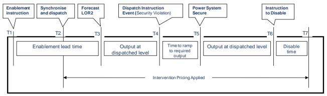
Enablement means preparing the *reserve equipment* to be *dispatched*. For example, Figure 1 demonstrates a fast response generator that does not need to be synchronised at the forecast LOR2 time (T2) to provide the reserve capacity. Note: a slow response generator may require *synchronising* and *loading* to its *minimum operating level* or some nominated level at the start of the LOR2 period (as shown in Figure 2), so that it can provide the reserve capacity within the timeframe required.
