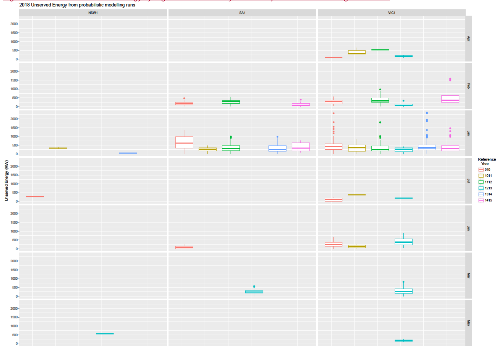
Figure 5: Variations in Unserved Energy by region and reference year across probabilistic modelling simulations
