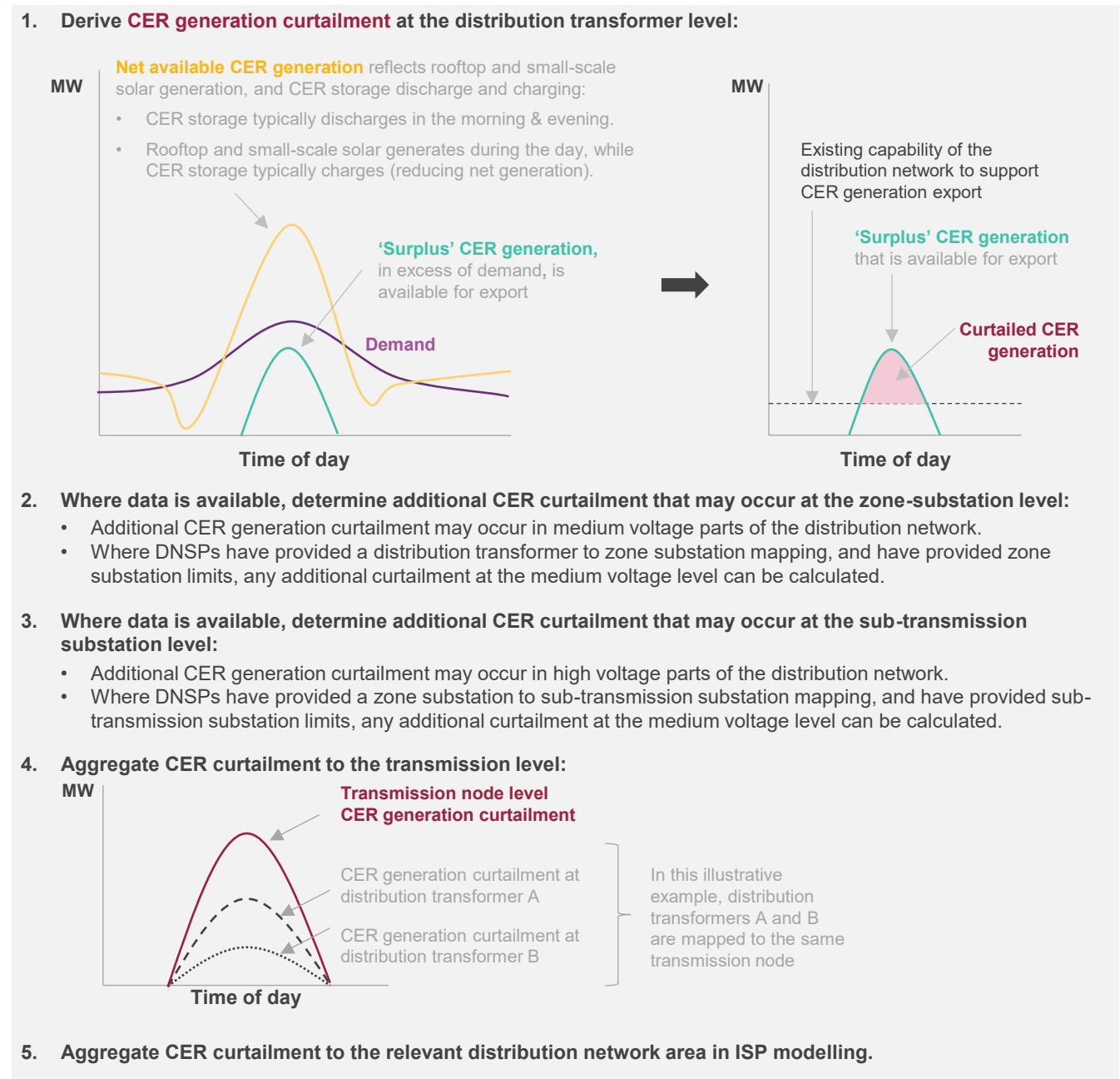
Figure 11 Illustration of the CER curtailment modelling under the LV Asset Data Template Pathway
