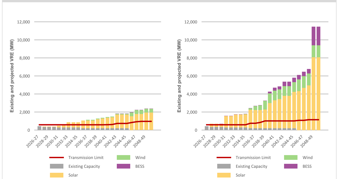
Transmission access expansion forecast for Step Change (left) and Accelerated Transition (right)
