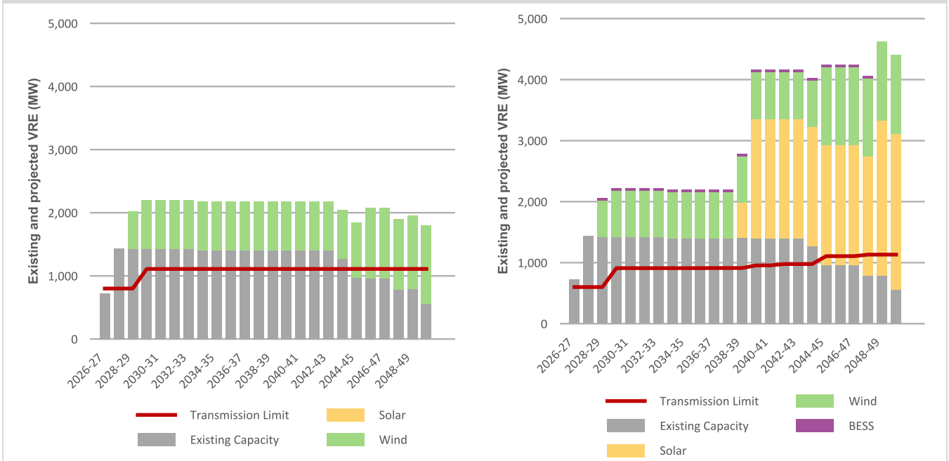
Transmission access expansion forecast for Step Change (left) and Accelerated Transition (right)
