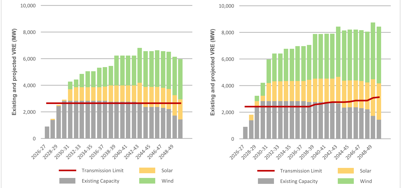
Transmission access expansion forecast for Step Change (left) and Accelerated Transition (right)
