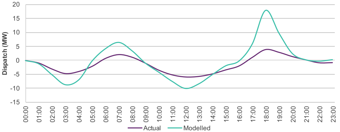
Figure 27 Actual and modelled average hourly dispatch profile of large-scale batteries in 2021-22 (MW)
