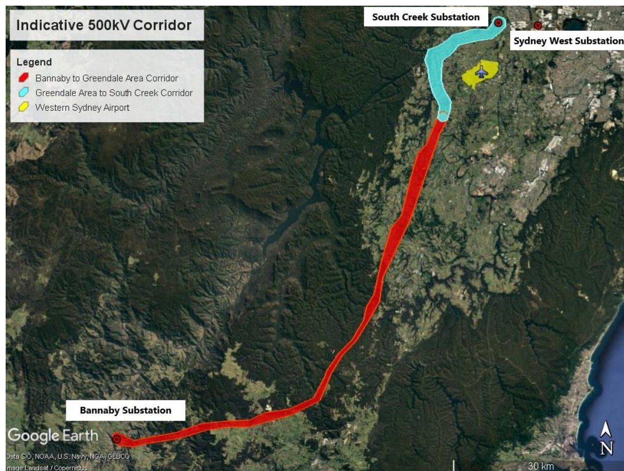
Figure 6 The indicative 500kV double circuit corridor for Sydney Southern Ring's preferred option
