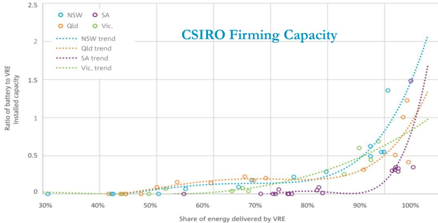
**Figure 11. Ratio of battery and VRE generation capacity (GW) required to achieve energy balancing for modelled shares of energy (GWh) delivered by VRE**
