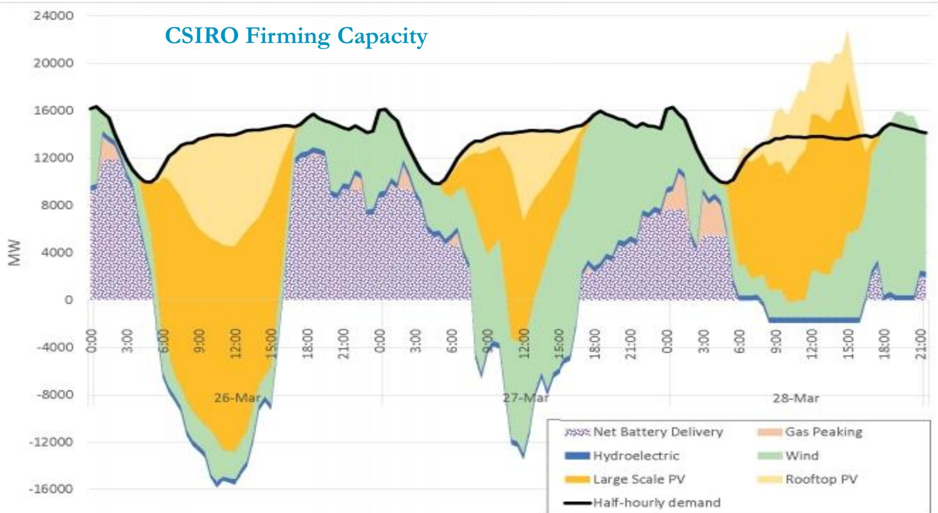
**Figure 37. Example time series of electricity supply and demand in Pathway 2 showing role of battery storage; NSW, 2046, 3 example days**
