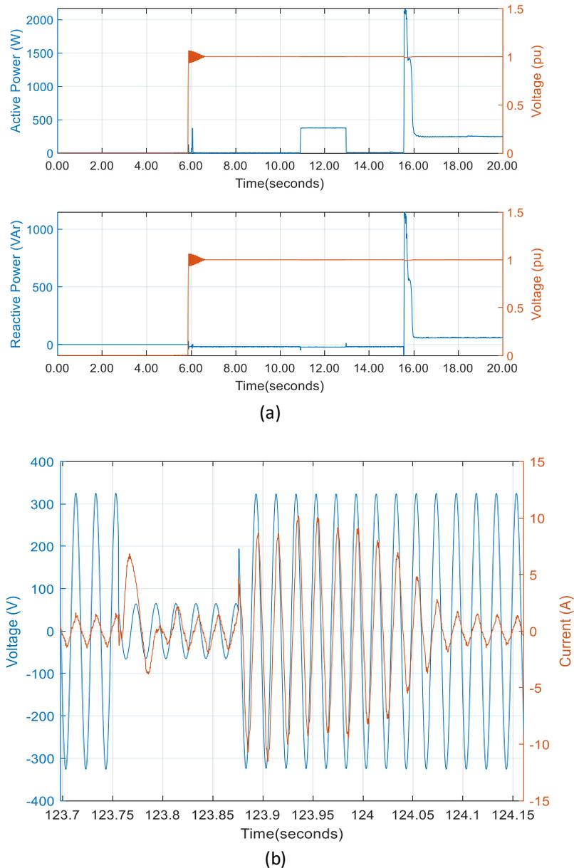
Figure 15: Results for Refrigerator Unit 3 (a) Device turn on behaviour (b) Inrush current for 0.2 pu sag for 120ms
