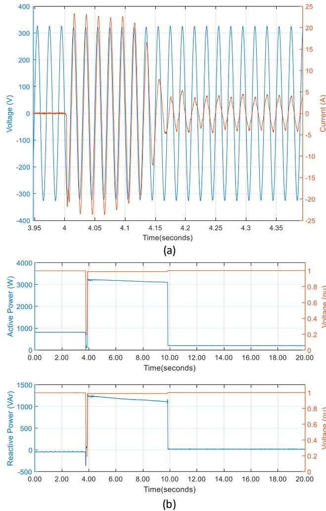
Figure 10: Results for Air Conditioner Unit 4 (a) Starting Transient (b) 0.2pu Sag for 120ms
