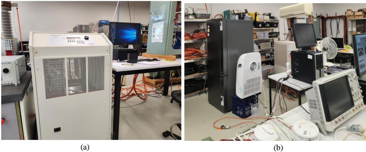
Figure 4: Load Testing Setup (a) Programmable Power Supply, and (b) Load under Test
