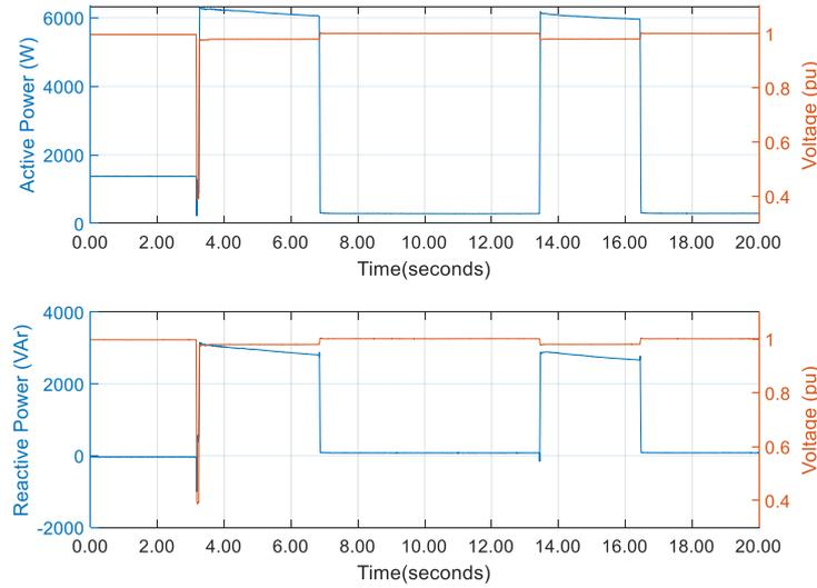
Figure 9: Response of Air Conditioner Unit 3 for 0.4 pu sag for 80ms
