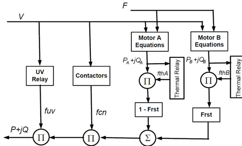
Figure 2: Motor D block diagram in the CMPLDW Model
