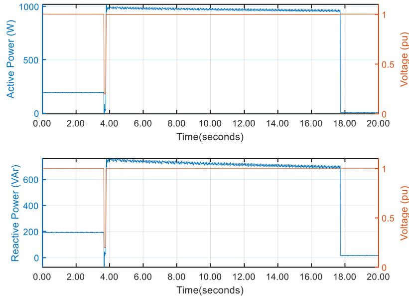
Figure 14: Stall and Disconnect Results for Refrigerator Unit 2
