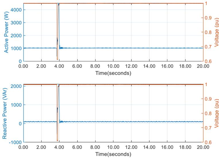
Figure 8: Detailed Sag Test for Air Conditioner 2
