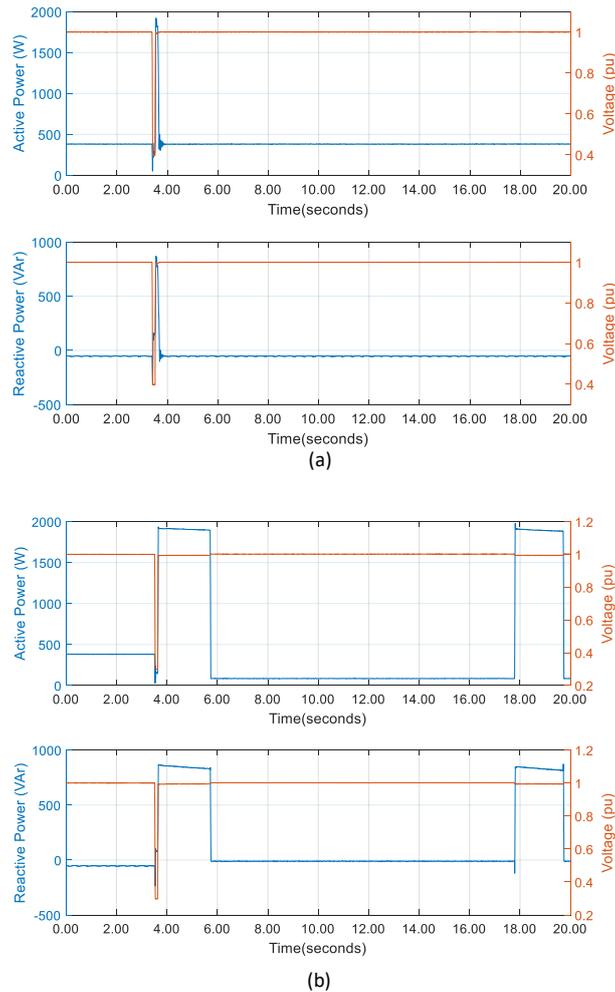
Figure 12: Response of A/C Unit 6 for a 120 ms Sag with retained voltage (a) 0.4pu (b) 0.3 pu
