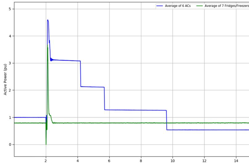
Figure 20: Aggregated response of ACs and Fridges for a 0.4 pu sag for a duration of 80ms
