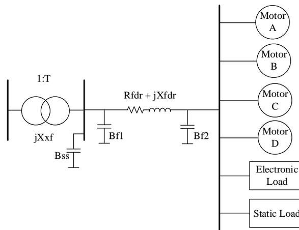
**Figure 1** WECC Composite Load Model Structure
