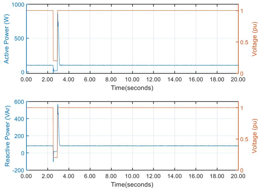
Figure 16: Refrigerator Unit 4 riding through extreme sag test
