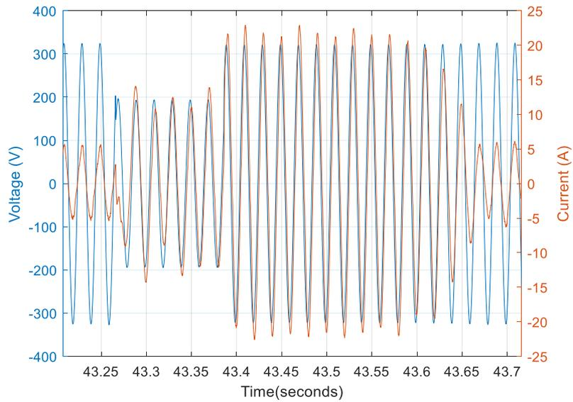
Figure 11 Response of Unit 5 for a 0.6 pu 120ms sag
