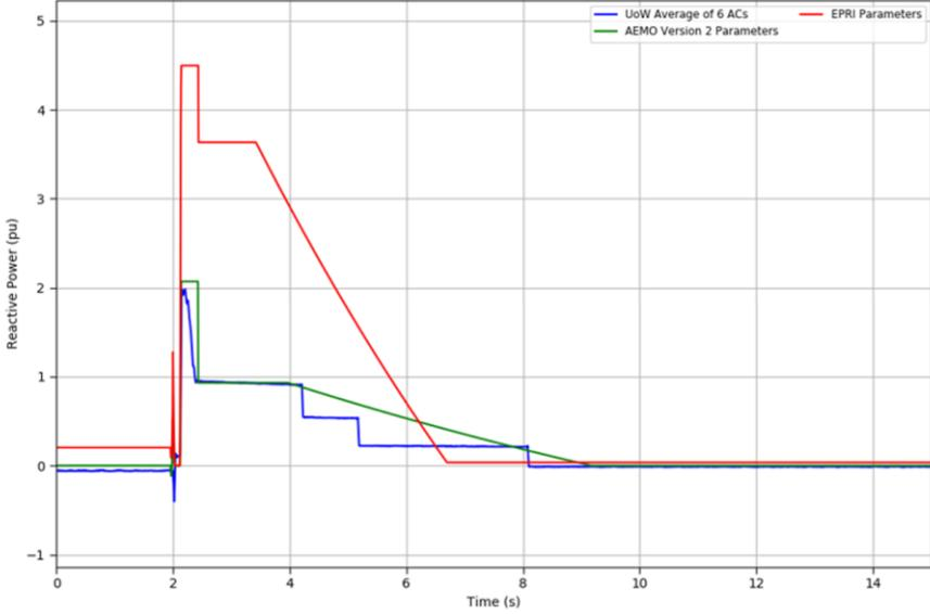
Figure 22: Reactive Power Response of Motor D with updated parameters
