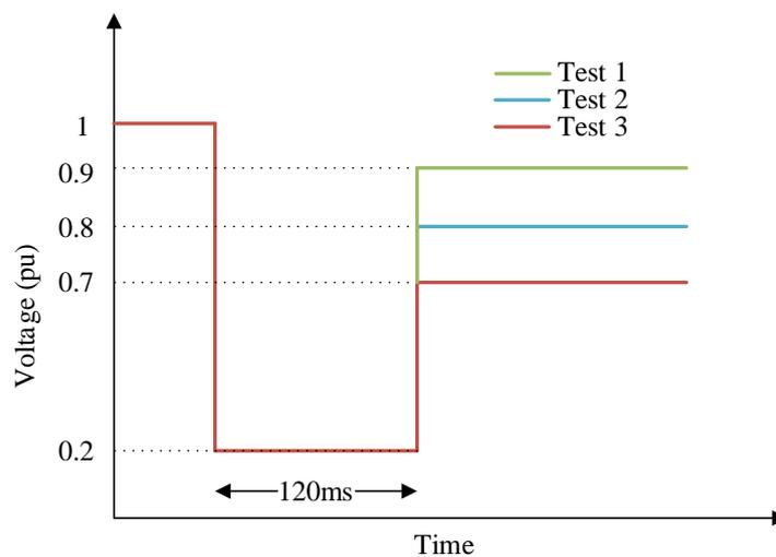
Figure 5: Tests done for Voltage Restart
