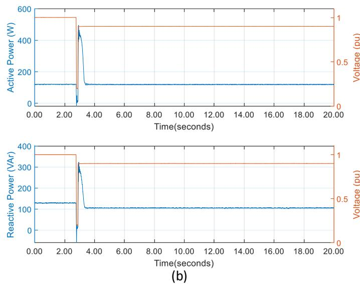
Figure 18: Freezer Unit 1 Results (a) Sag for 120ms at 0.2 pu (b) Voltage Restored to 0.9 pu
