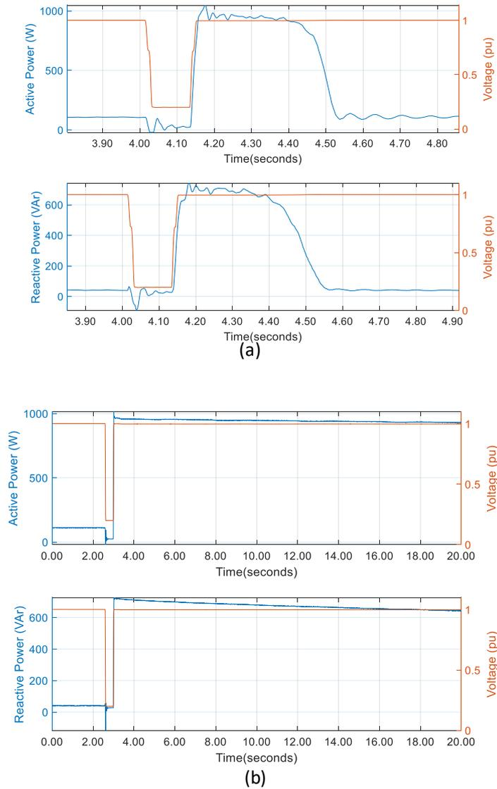
Figure 13: Results for Refrigerator Unit 1 (a) Stall and Restart for 0.2 pu Sag for 120ms (b) Extreme Sag Test Response
