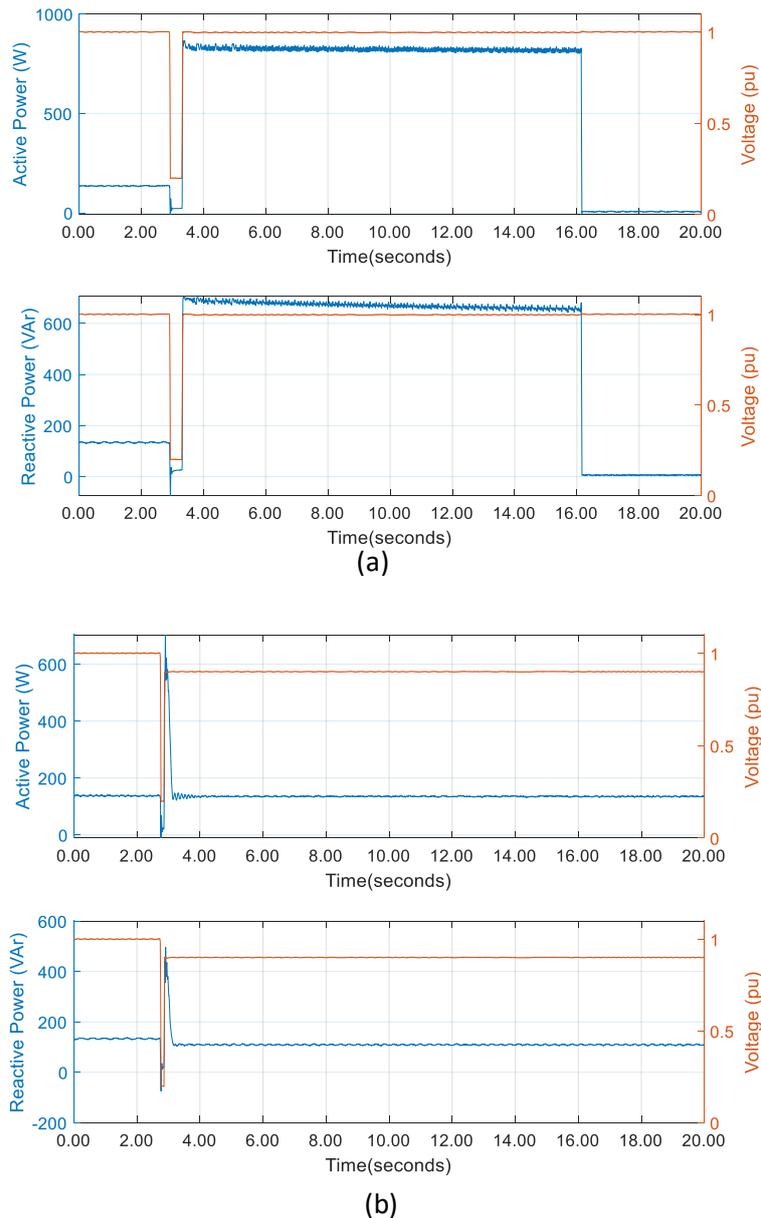
Figure 17: Results for Refrigerator Unit 5 (a) Extreme Sag Test (b) Voltage Restart Result
