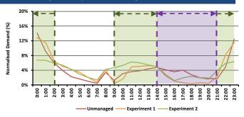
Source: Origin, Energeia Analysis. Note: Unmanaged: 13 vehicles, Exp 1: 13 vehicles, Exp 2: 13 vehicles. Green indicates incentive to charge, purple indicates controlled charging (Experiment 2 only)
