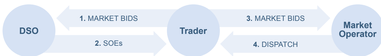
Figure 3. Market bids first sent to the DSO to create shaped operating envelopes.
