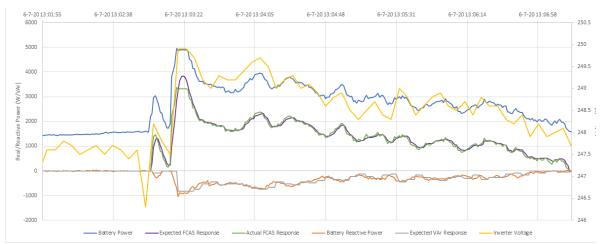
Figure 8 Coincident volt-var and contingency FCAS response from an FCAS-enabled VPP site
