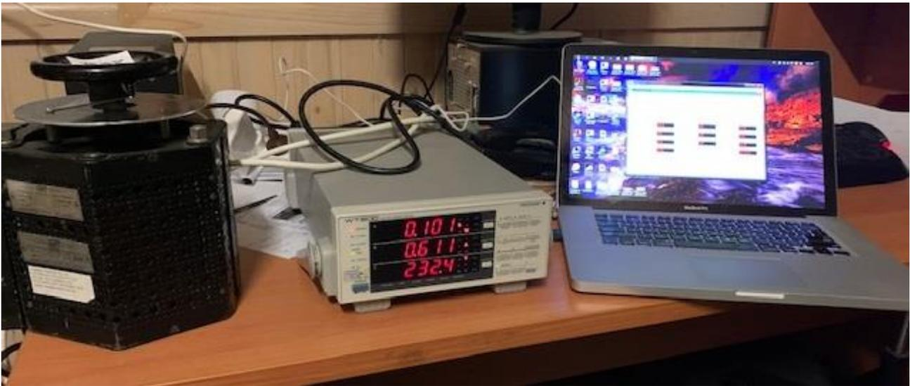
**Figure 1: Equipment used to measure electrical characteristics at low voltage**
