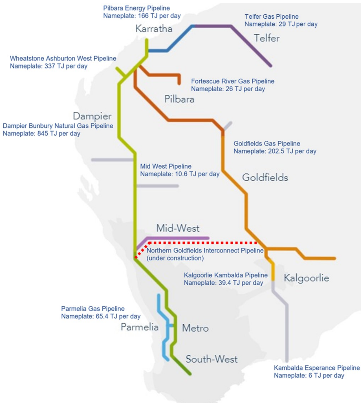
Figure 4 Gas transmission pipelines in WA
