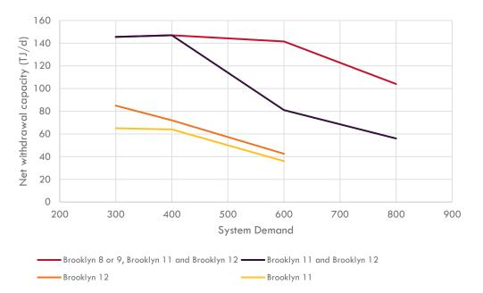
Figure 19 Net withdrawal capacity with Brooklyn CS reconfiguration and Winchelsea CS bi-directional
