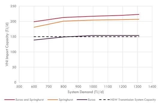
Figure 21 Victorian Northern Interconnect import capacity post VNI Expansion (VNIE) Phase B project
