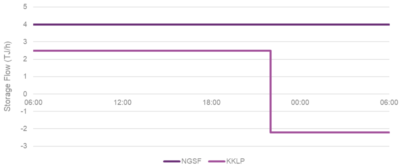
Figure 21 Modelled storage injections from Newcastle Gas Storage Facility and Kurri Kurri Lateral Pipeline (TJ/h)
