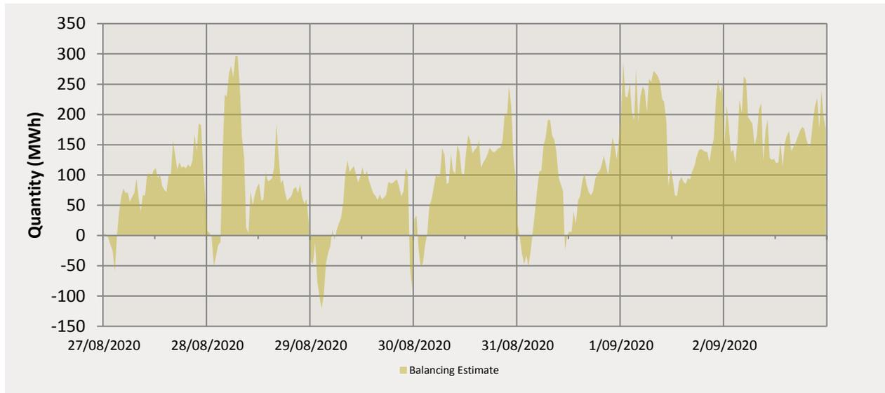
The majority of the balancing activity this week occurred within Balancing Demand. The maximum balancing demand for the week reached 296.6965 MWh on the 28/8/2020. The maximum balancing supply for the week reached -121.048 MWh on the 29/8/2020.
