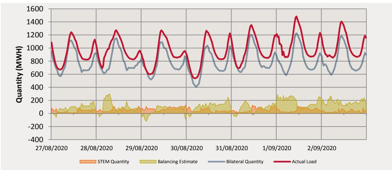
Total balancing supply equalled -1299.699 MWh whereas total balancing demand equalled 37821.035 MWh. The Total STEM Traded quantity was 16825.697 MWh, with the STEM Clearing Quantity ranging between 4.45 MWh and 128.227 MWh.
