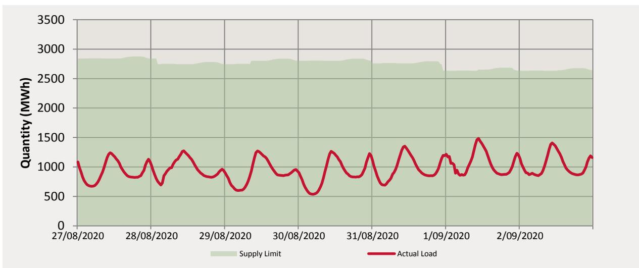
The supply limit ranged from 2632.338 MWh to 2874.907 MWh
