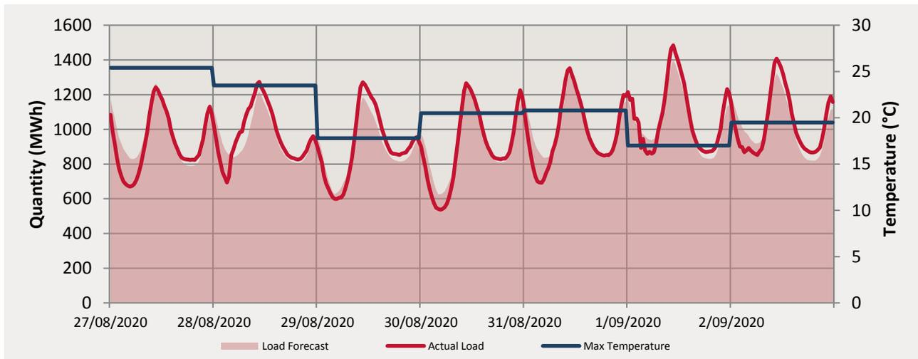
The maximum temperatures for this trading week ranged from 17°C to 25.4°C. The actual load peaked at 1484.054 MWh on the 1/9/2020.
