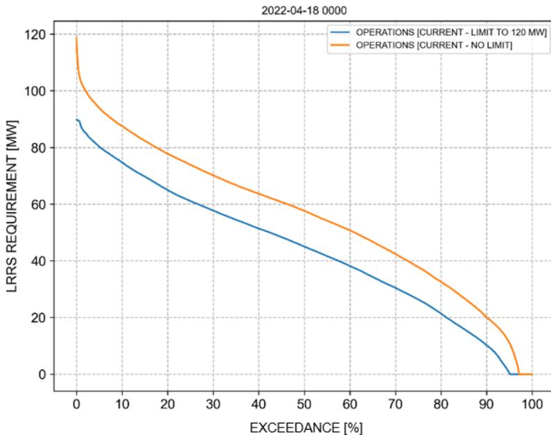
As seen in Figure 7, the increased EGF power transfer resulted in a higher maximum dynamic LRR requirement. When comparing the dynamic LRR requirements before and after the increase, the new requirement was within 90MW for 93% of the time of the analysis period.
