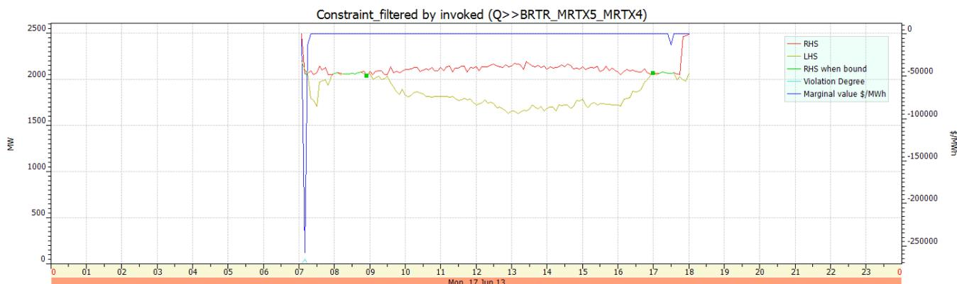
The period that is most interesting is the period leading up to 5pm. In this period the outage resulted in SWQ generation being constrained off as Braemar increased dispatch (Braemar adds to the flow through the flowgate), and displaced the QNI interconnector, resulting in SWQ generators and the interconnector no longer being able to set the RRP and the price plant not in the flowgate. This is shown in figure 3.
