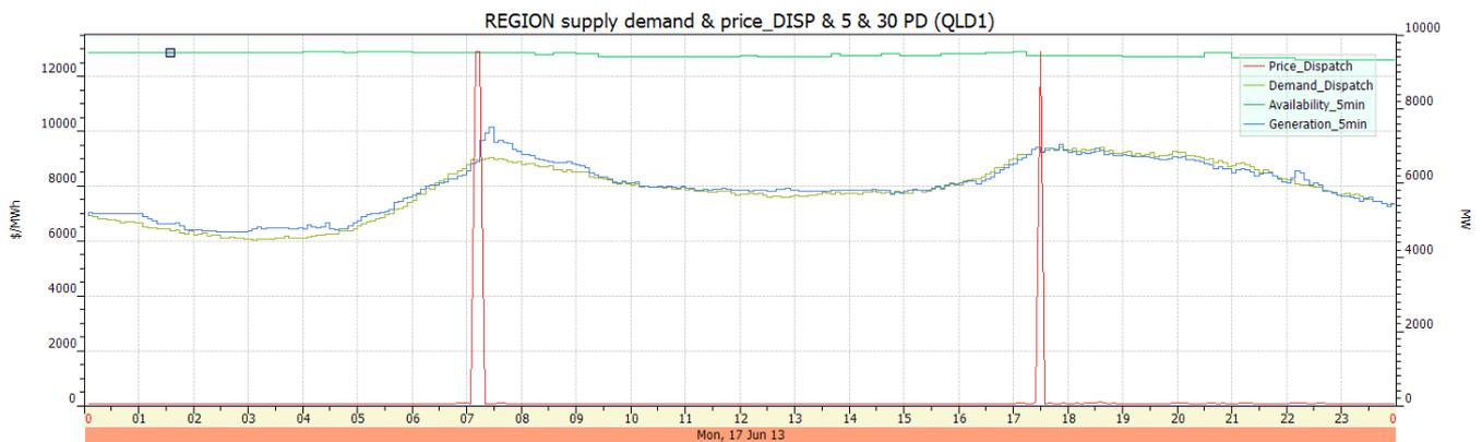
The high prices were reflected in the marginal values of the constraint equation, which were exacerbated because, when the outage was taken, AEMO introduced a constraint equation that could not be satisfied and therefore “violated”. This can be seen in Figure 2.
