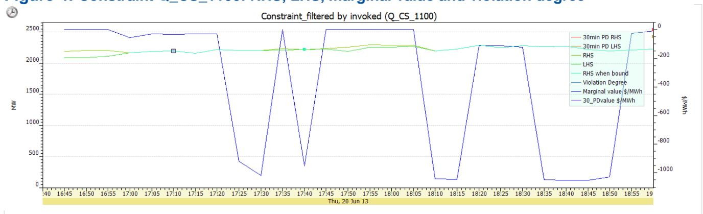
In order not to be constrained off those north on the sending end of the looped constraint could price down to  $-\$1,000/\text{MWh}$  to maintain dispatch (see below), but this was complicated by a 'Feeder Bushing' constraint which principally constrains off Gladstone, but under the outage conditions of Calvale-Halys included all generation in Central-North QLD (as these generators had less flow allowed through the other flowgate and therefore had more flow through another flowgate).
