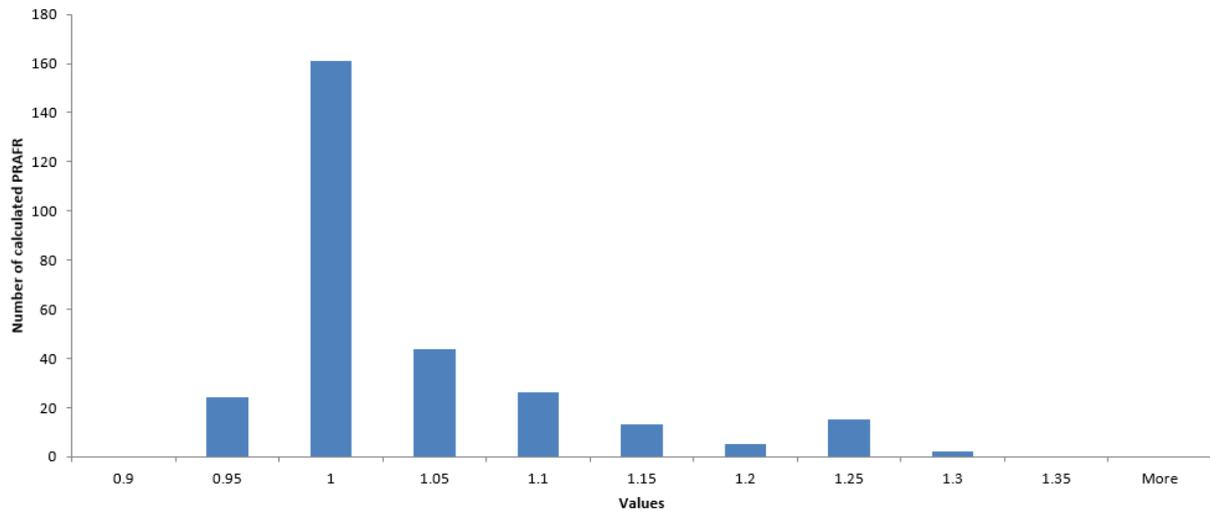
The results from analysing distribution of PRAF values for both load and generation are as expected. This indicates that calculation of PRAFRs for both load and generation are generally working as intended.
