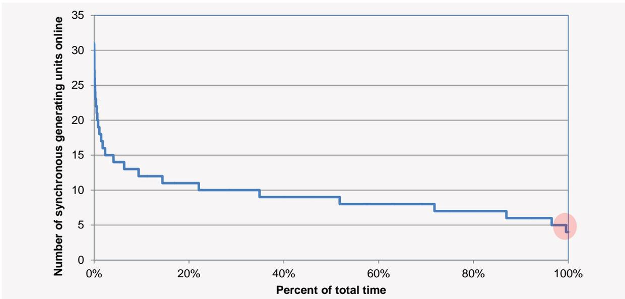
Synchronous generators provide services to the power system such as inertia, frequency control capability, reactive support, and fault level for riding through power system disturbances. These support system security, and they reduce or disappear as synchronous generation is displaced from the power system by non-synchronous renewable generation.
