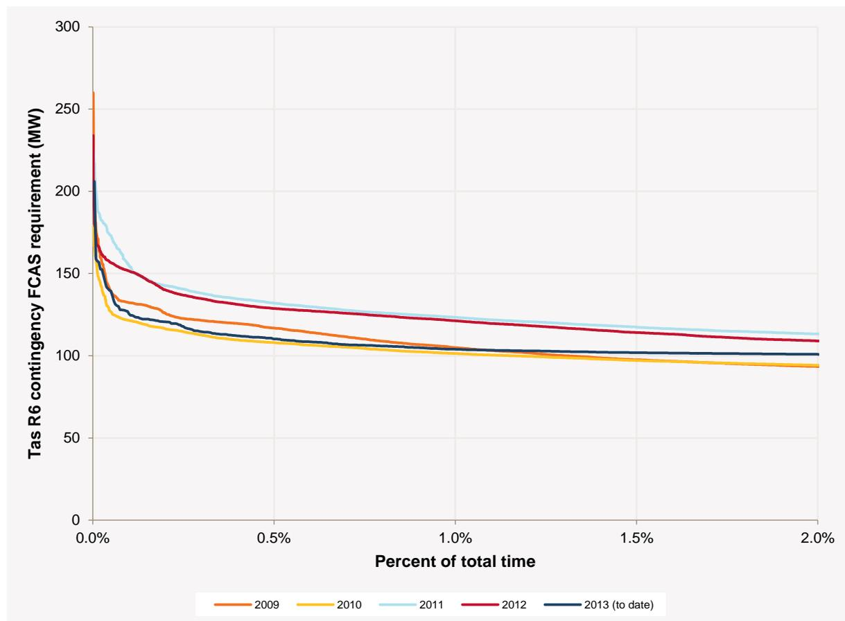
Transend and AEMO are currently reviewing the calculation used to determine contingency FCAS requirements in Tasmania, due to the service of Musselroe Wind Farm. This review suggests the need to update this calculation to better consider the fault ride through behaviour of both Tasmanian wind generation and Basslink, and the behaviour of the Basslink Frequency Controller. Further information on these issues is provided in sections 3.6.8 and 3.4.1.
