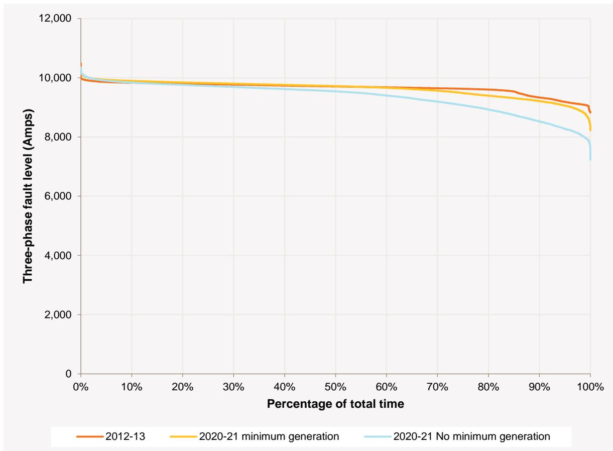
**Figure 7-13 — Simulated Hazelwood 220 kV Bus 3/4 fault levels**
