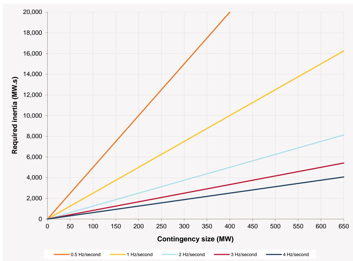
Assuming an allowable system RoCoF range of between 1 and 4 Hz/s:
