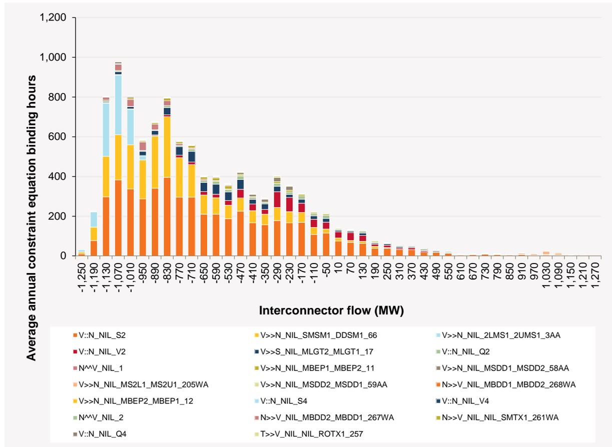
This chart shows that the constraint equation V::N\_NIL\_S2 limited interconnection flows and wind farm output for a combined total of 5,062 hours in 2020–21. This is almost double the duration seen when new wind generation was excluded from these stability constraints.
