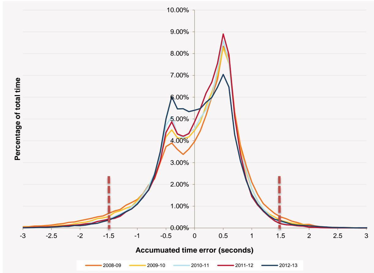
Installed wind generation capacity in the NEM increased from around 1,100 MW to 2,500 MW in the five-year period covered by this data. Figure 3-8 does not indicate any increase in the accumulated time error on the mainland during this period, and in fact shows a slight reduction.
