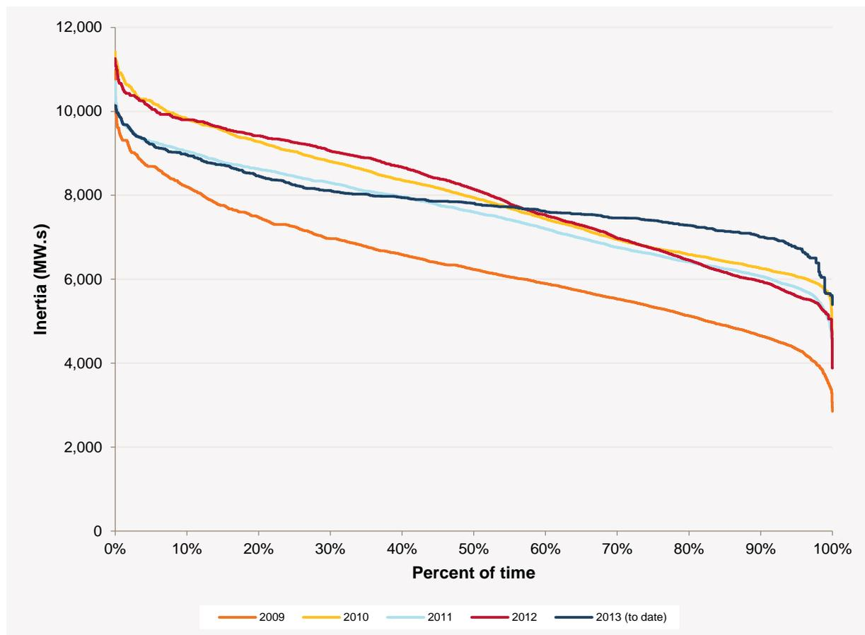
The increase in power system inertia seen in Tasmania after 2009 is mainly due to the commissioning of the Tamar Valley Combined Cycle Gas Turbine in that year; this generation type has relatively high inertia and it has operated with a high capacity factor since commissioning.
