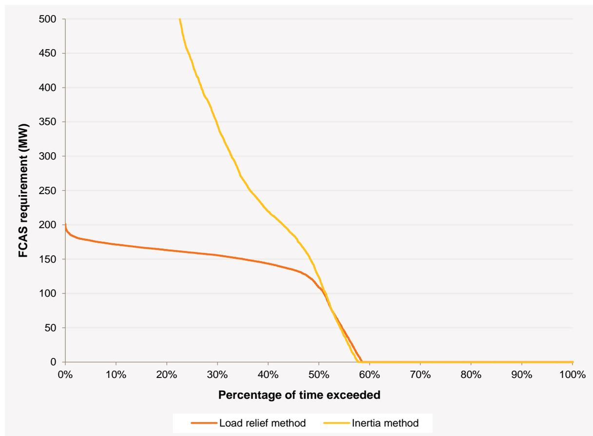
Figure 7-6 shows that for the majority of conditions where South Australia was required to obtain local L6 contingency FCAS, the more accurate requirement calculated considering power system inertia is higher than that calculated only considering frequency dependent load relief.
