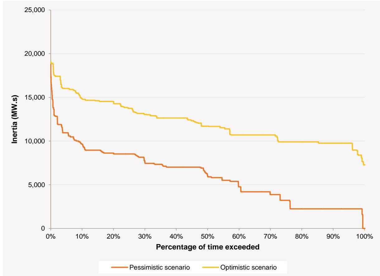
This figure shows the impact of rigidly maintaining minimum output levels from existing synchronous generation. An inertia increase of up to 8,000 MW.s is seen in the optimistic high-inertia scenario, compared to the pessimistic, low-inertia scenario, where wind is dispatched ahead of all other forms of generation.
