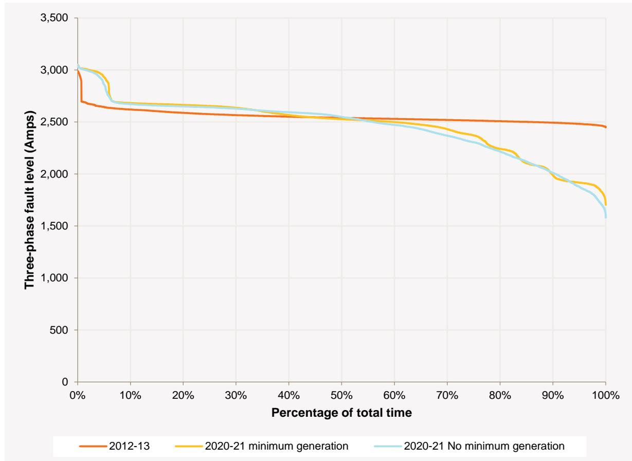
The 2012–13 and 2020–21 simulations with minimum generation limits produce fault levels that are well within (and at the higher end of) the ranges indicated by Transend’s APR.
