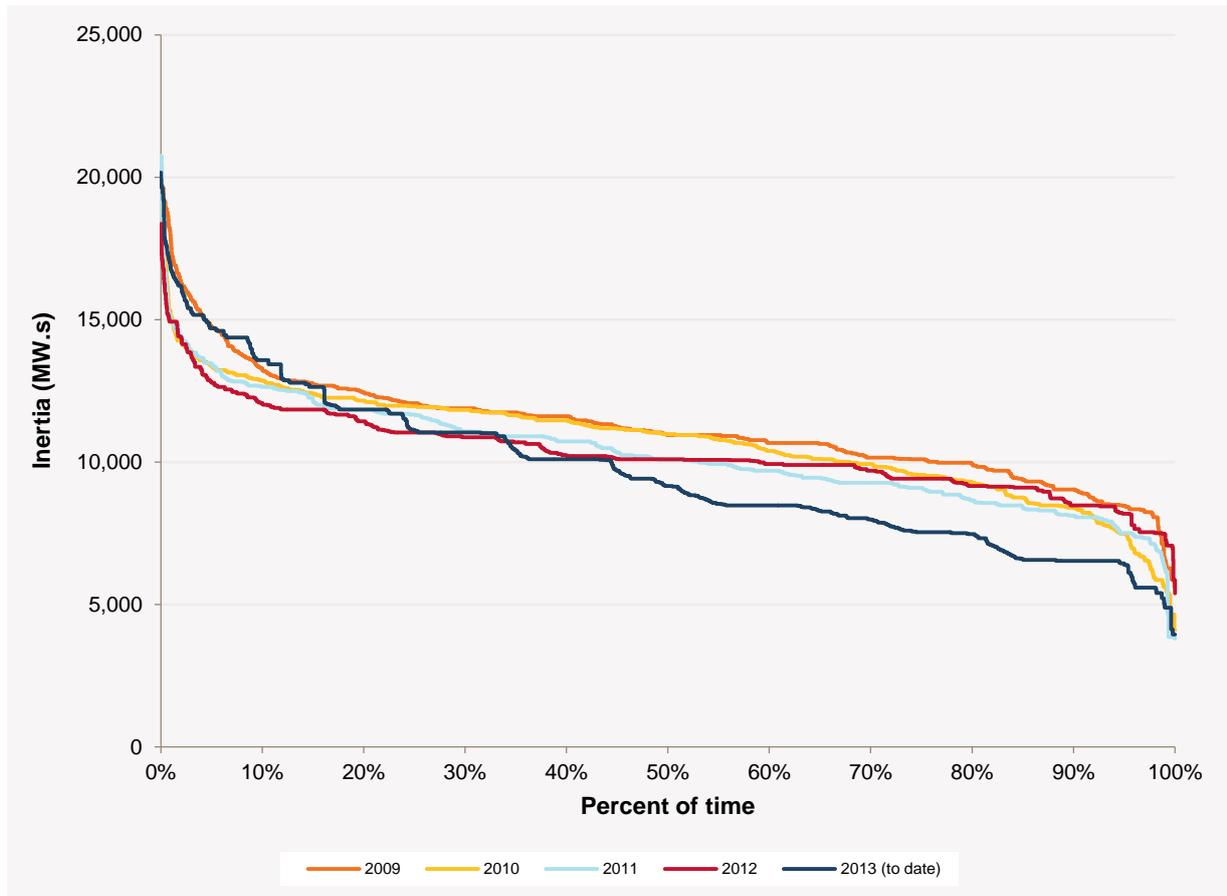
The reduced power system inertia seen in South Australia until late May 2013 is due to the shutdown of both units at Northern Power Station. Unit 1 was out of service from late April, and Unit 2 was out of service from late March. The combined inertia of these two generating units (3,000 MW.s) represents a material proportion of the typical power system inertia in South Australia.
