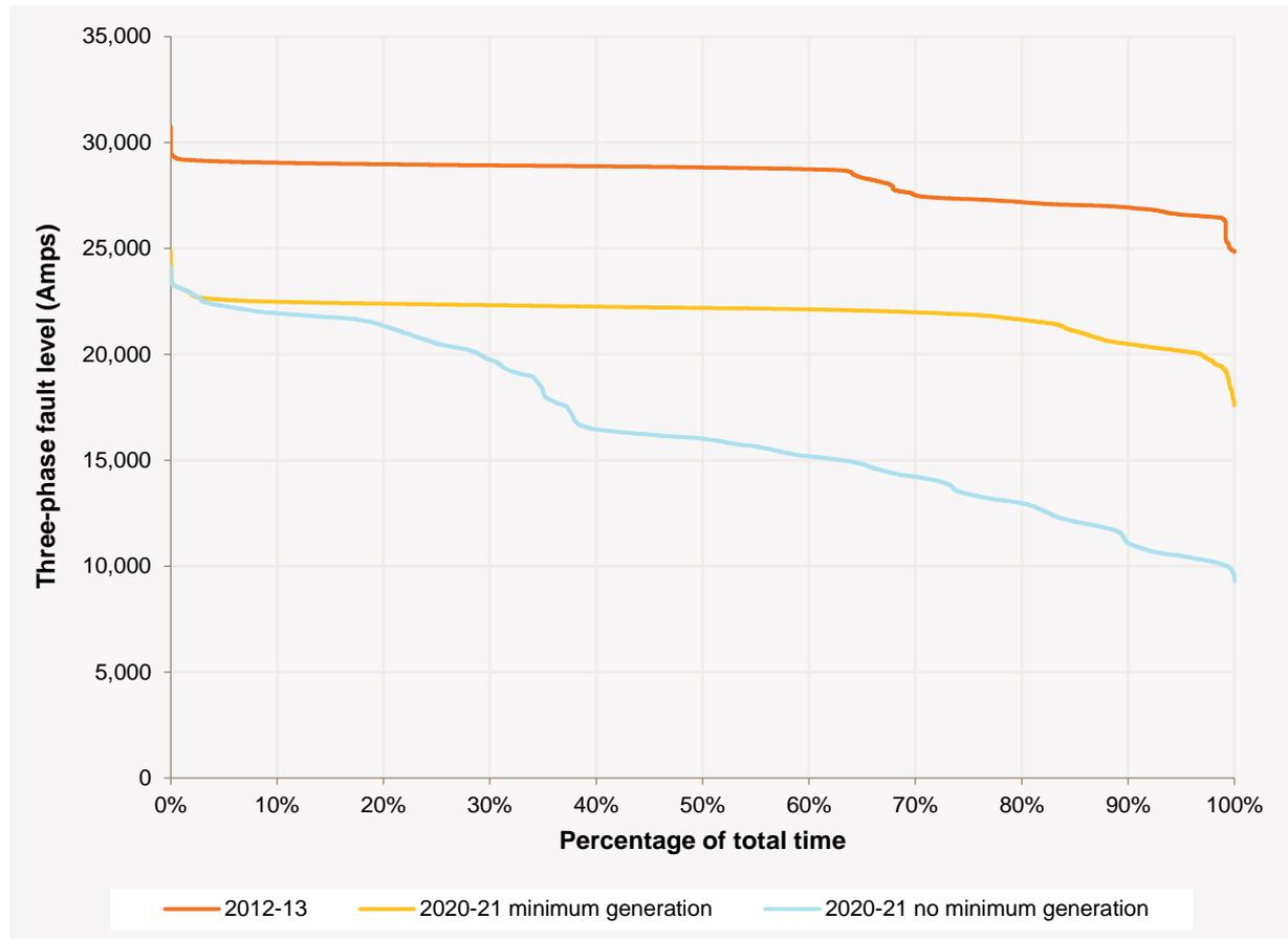
These studies again suggest that the largest variations in fault levels will occur for electrical connection points close to large amounts of synchronous generation. Fault levels calculated for electrically strong busses, such as Hazelwood in the Victorian Latrobe valley, are sensitive to generation levels.
