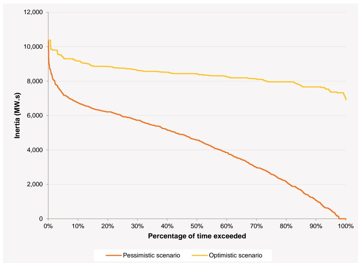
This figure shows the impact of rigidly maintaining minimum output levels from the existing synchronous generators in market modelling (optimistic scenario). This modelling results in inertia increases of up to 7,000 MW.s compared to cases where wind is dispatched ahead of other forms of generation.
