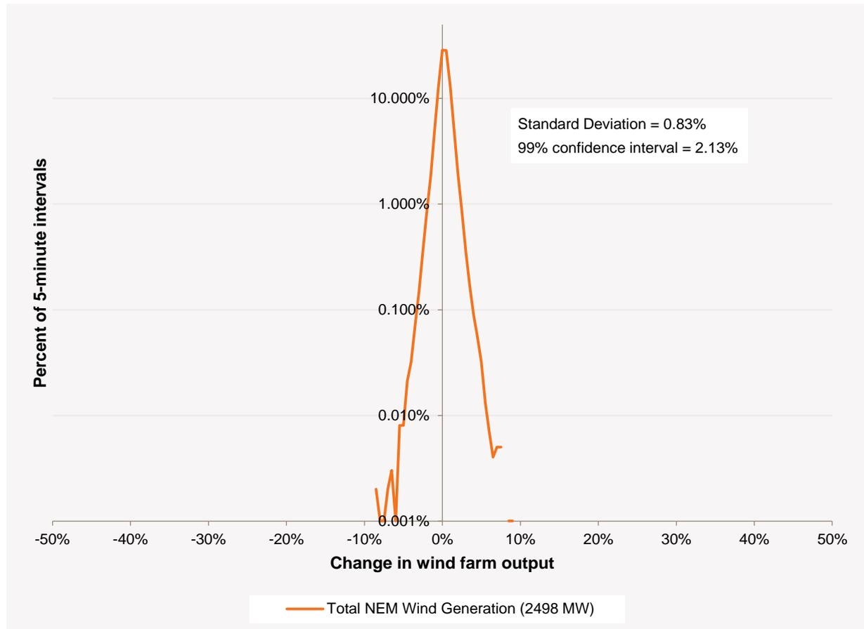
A key point evident in these figures is that the aggregate wind generation output, both within a region and across the NEM, changes less (as a percentage of installed capacity) over a five-minute period than the output of any single wind farm. The standard deviation of the distribution of five-minute changes becomes smaller as wind generation capacity is installed over a larger geographical area.
