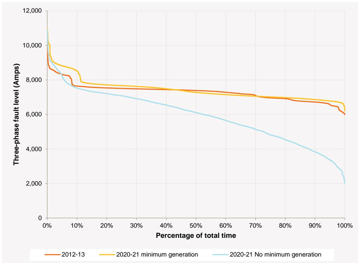
**Figure 7-9 — Simulated Derby 110 kV fault levels**
