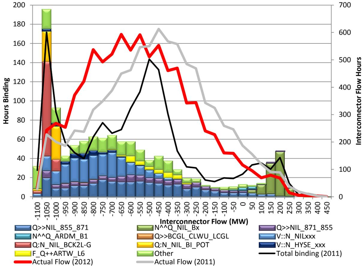
Figure 15: Binding constraint equation distribution for NSW1-QLD1
