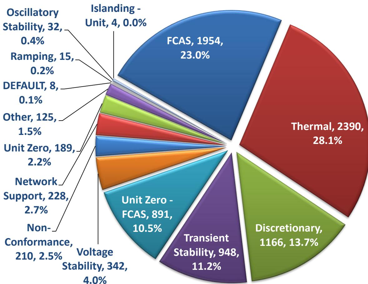
Figure 2: Constraint equations by limit type
