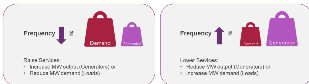
Figure 1 Impact of supply/demand balance on frequency
