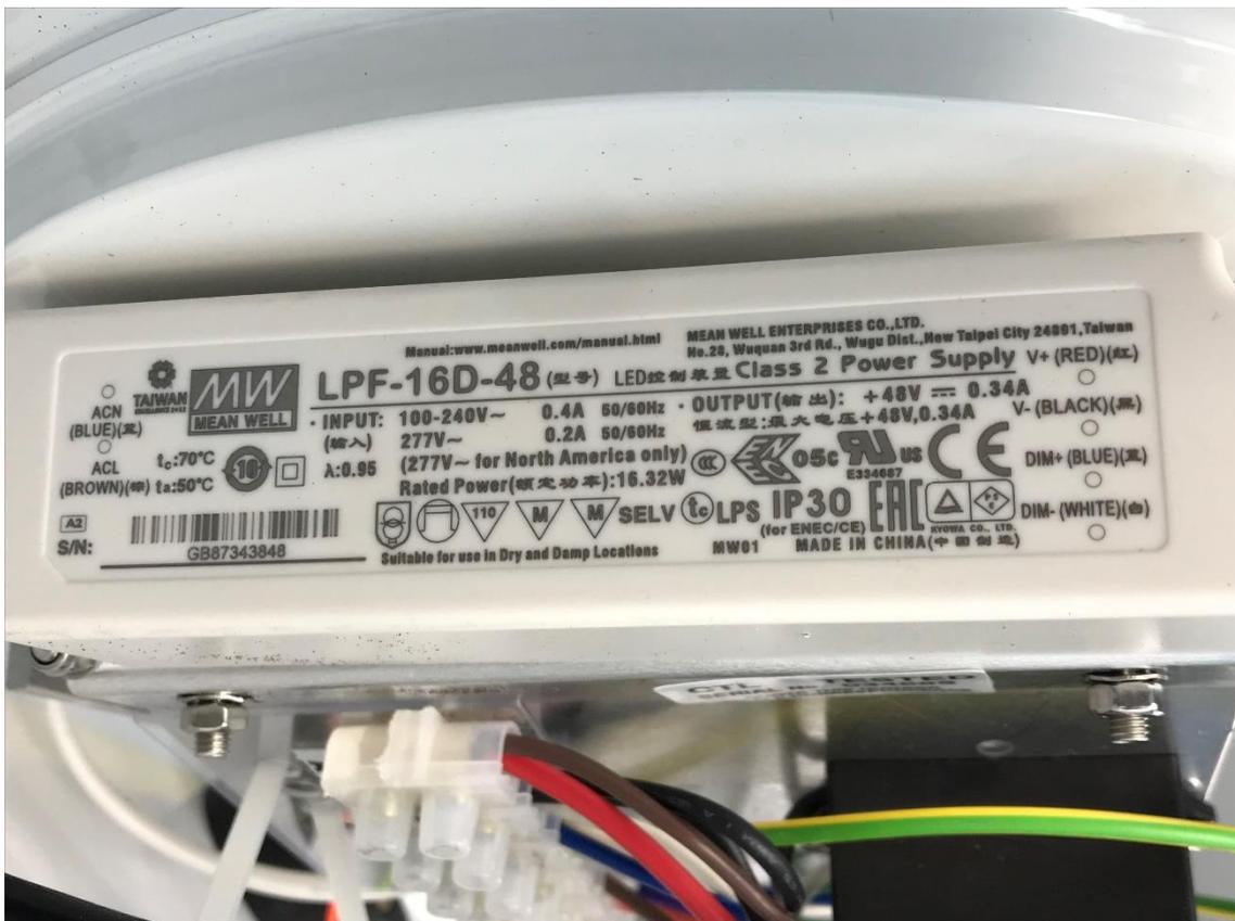
Rating label for LED control gear
