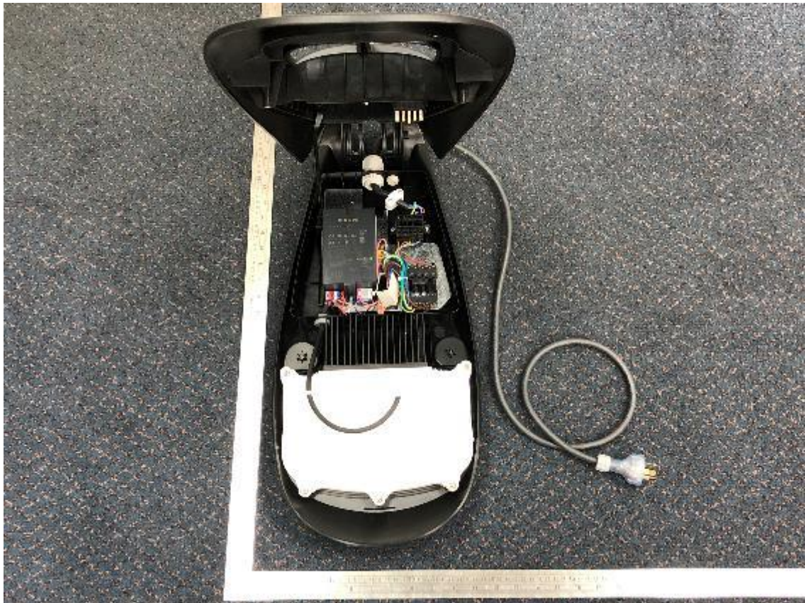
25W luminaire model – Internal construction
