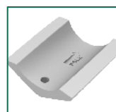
5° Tilt Adjustment Adapter for Spigots. Ensures that correct tilt can be achieved if the original pole outreach angle is incorrect. Factory fitted. Can in some instances be site fitted.
