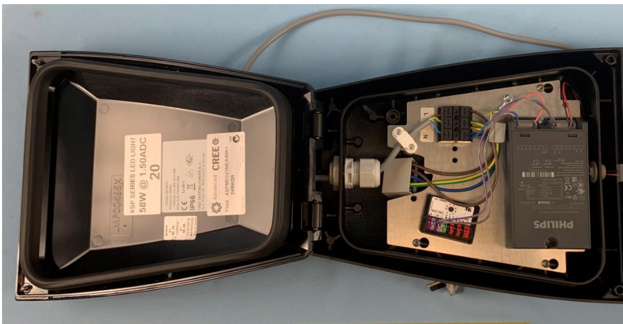
Model XSPME023MEA40K+24BKQ9; XSPME023MEA40K+24BKQ6; XSPME023MEA40K+24BKQ2 - Internal construction
