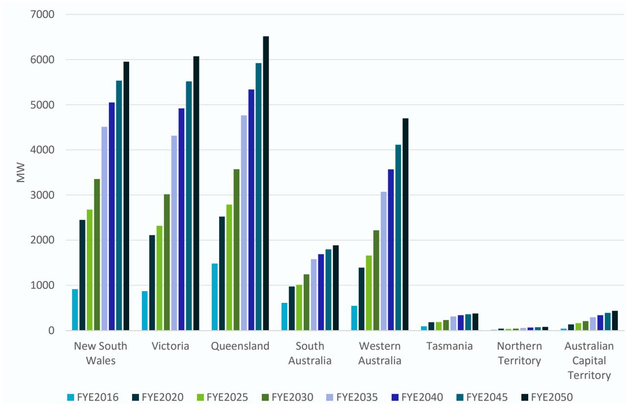
Figure 5-2: Projected effective residential rooftop solar capacity by state under the Moderate scenario
