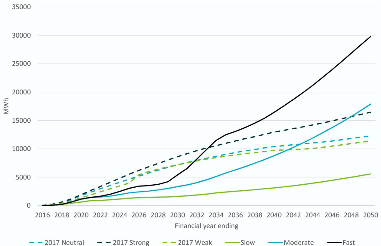
**Figure 5-8: Projected residential battery storage capacity by scenario compared with 2017 scenario projections**
