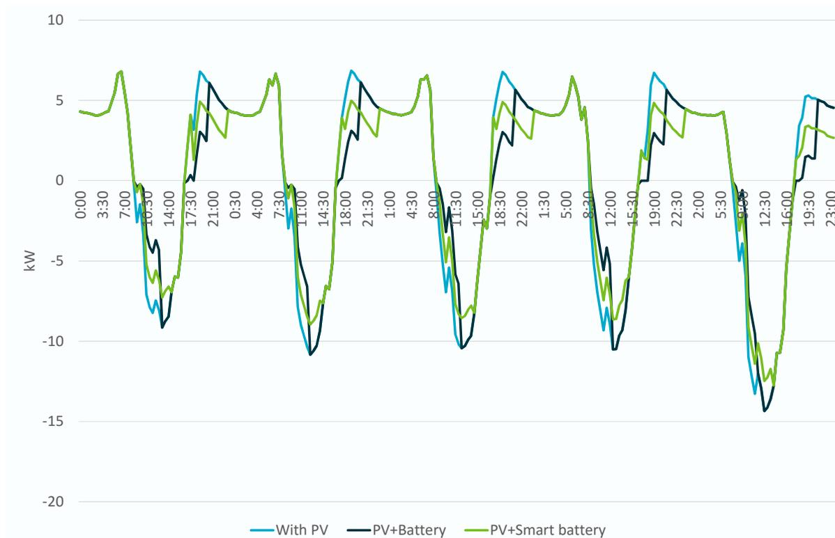
**Figure 5-23: Sample of commercial load during summer under two battery management regimes**
