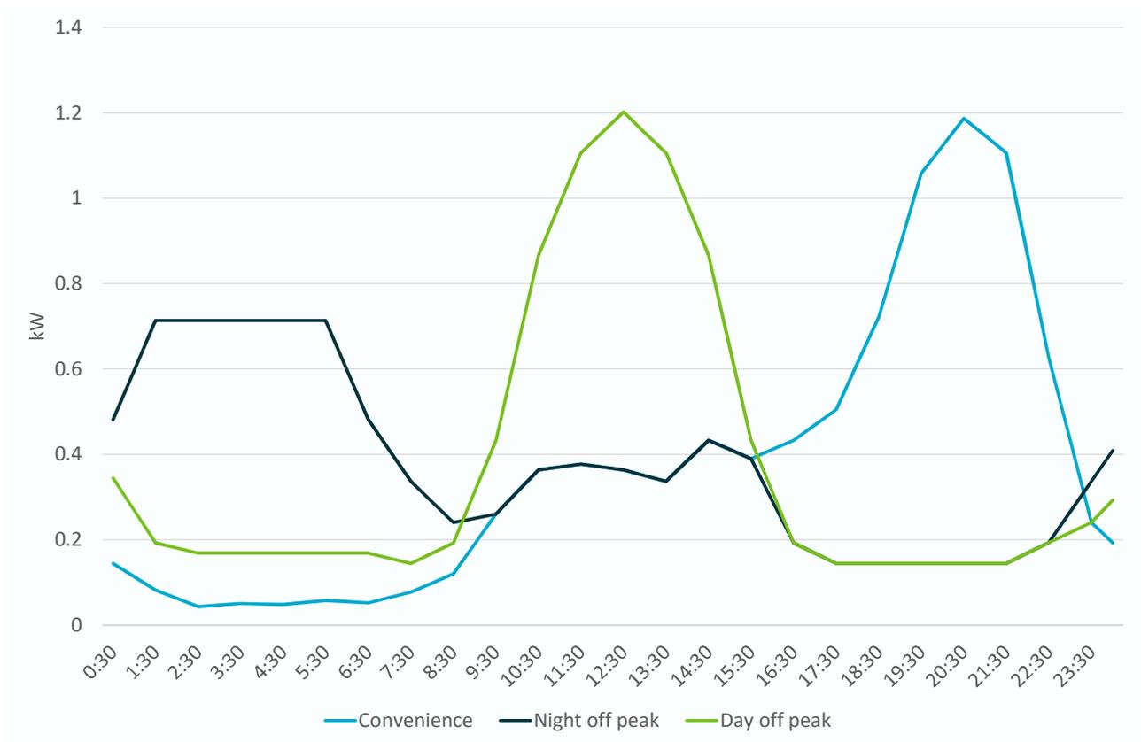
Figure 5-19: Electric vehicle charging profiles for passenger (residential) vehicles
