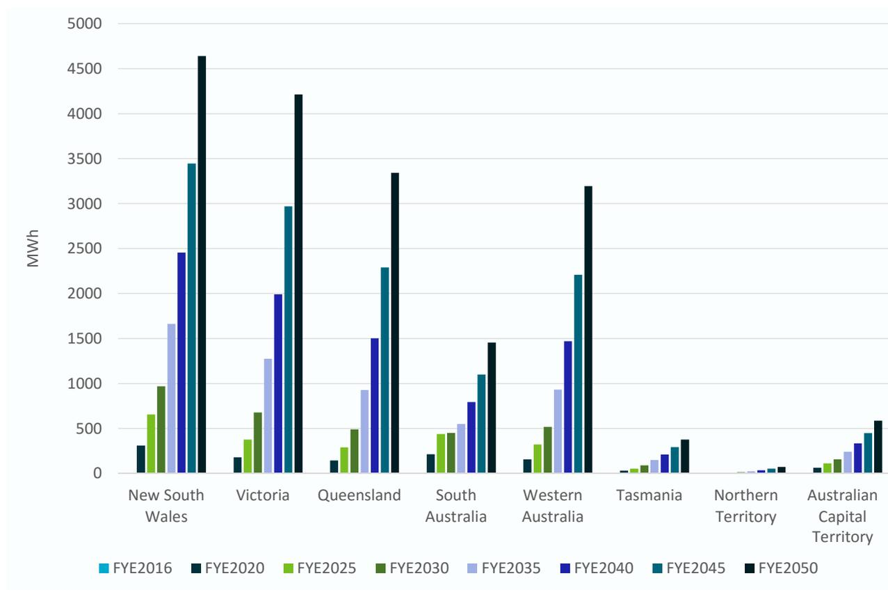
**Figure 5-9: Projected residential battery capacity by state under the Moderate scenario**
