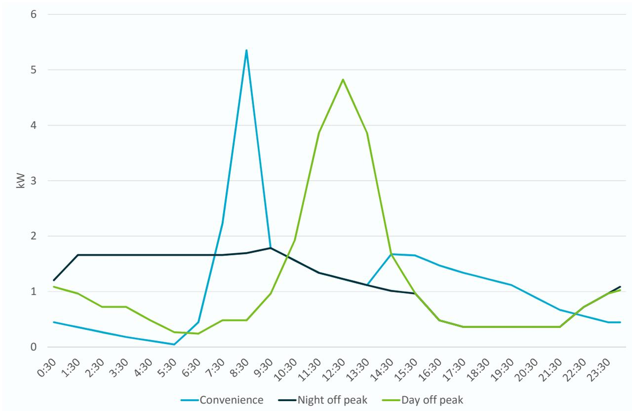
Figure 5-21: Electric vehicle charging profiles for trucks and buses (heavy commercial) vehicles
