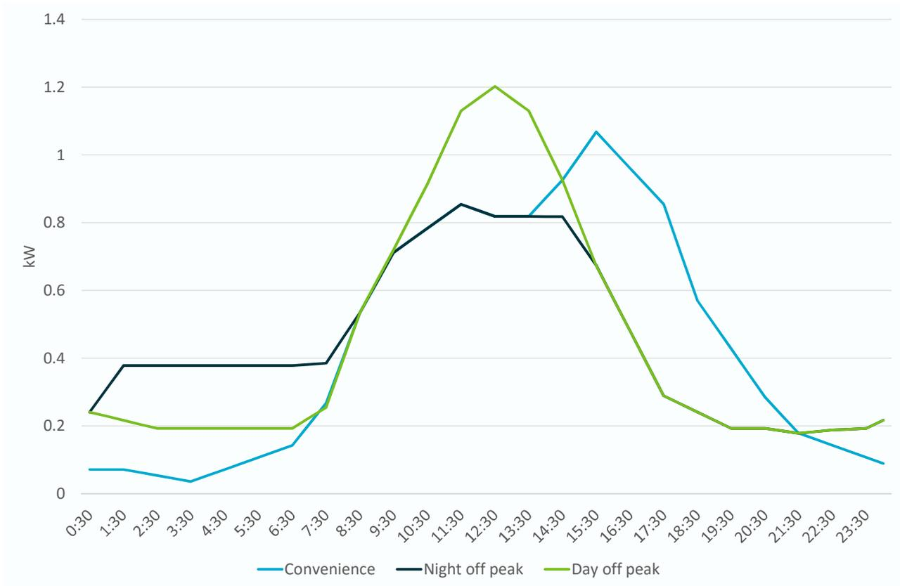
Figure 5-20: Electric vehicle charging profiles for light commercial vehicles
