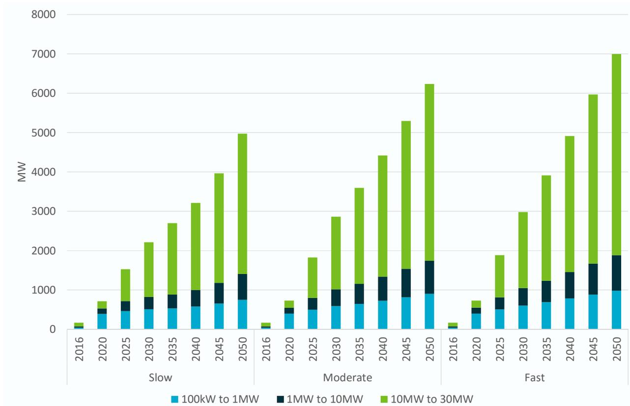
**Figure 5-6: Breakdown of projected effective commercial non-scheduled solar generation capacity by capacity size and scenario**
