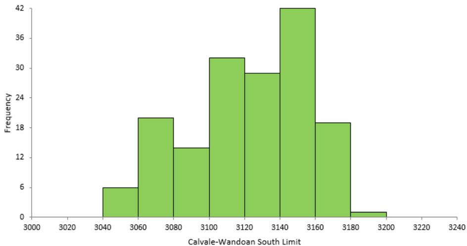
**Figure 4 – Histogram of calculated transient stability limits across CQSQ**
