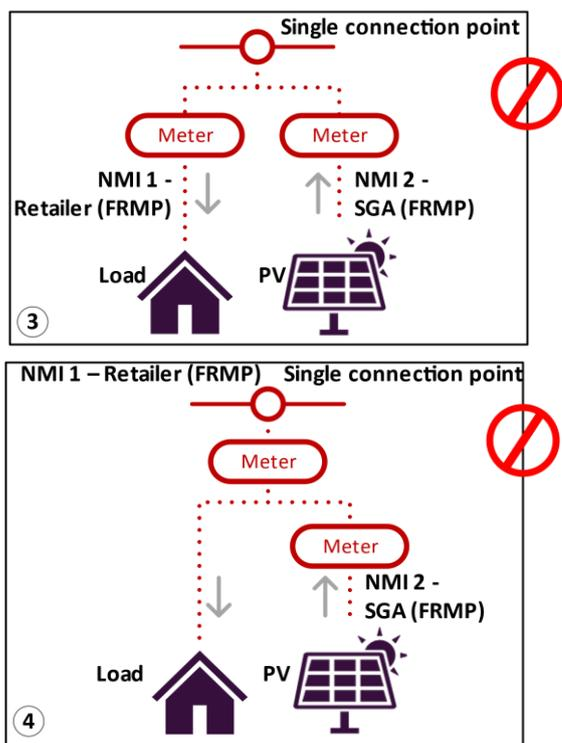
**Figure 1 SGA Configurations**
