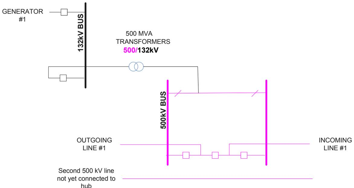
Figure 11: Stage 1 of 500/132 kV Hub for Connecting Generating Capacity in the Range of 0 MVA - 500 MVA
