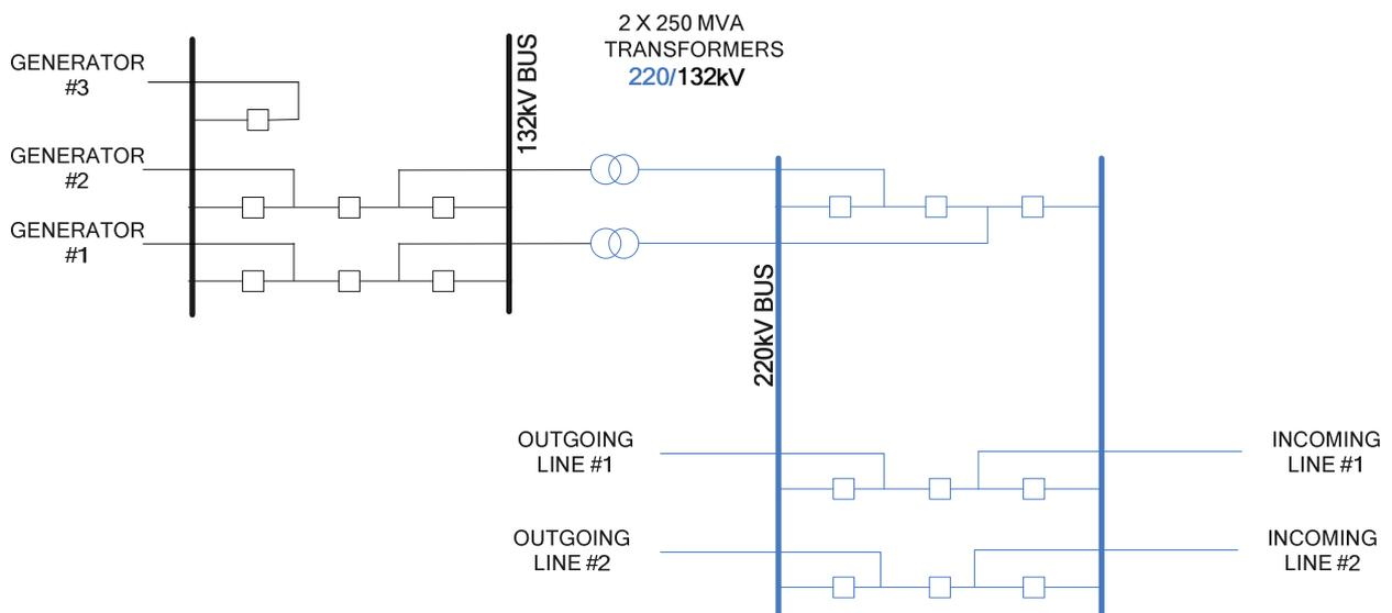
Figure 9: Stage 2 of 220/132 kV Hub to Connect Generating Capacity in the Range 250 MVA - 500 MVA
