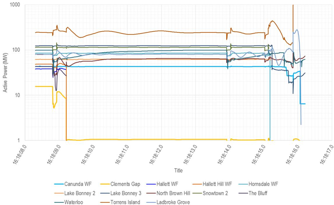
The measured values for generator active power are shown in Appendix I. Comparisons of measured and simulated response of each generating system are presented in Figure 122 to Figure 131. Note that PSS/E dynamic simulation could not be continued after 16:18:16, due to inability of the dynamic simulation solver to deal with rapidly changing dynamics.
