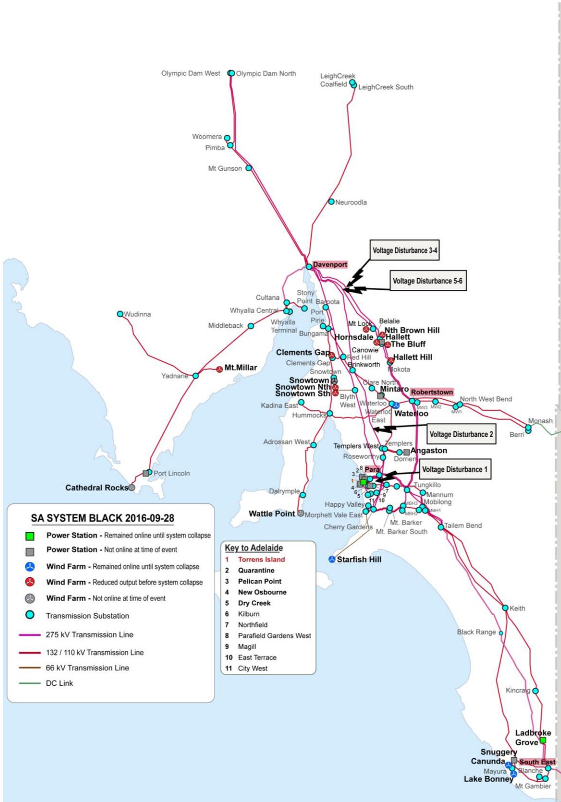
Five transmission line faults, resulting in six voltage disturbances on the network, caused sustained loss of power from multiple generating systems. This, in turn, initiated a sequence of events that ultimately led to the Black System. Table 7 provides more detail on each transmission line fault.
