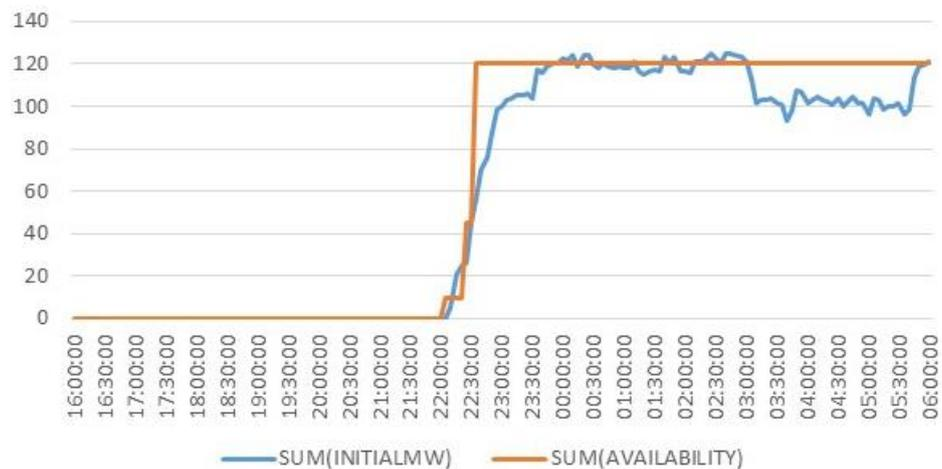
**Figure 115 Pelican Point Power Station MW output during restoration**
