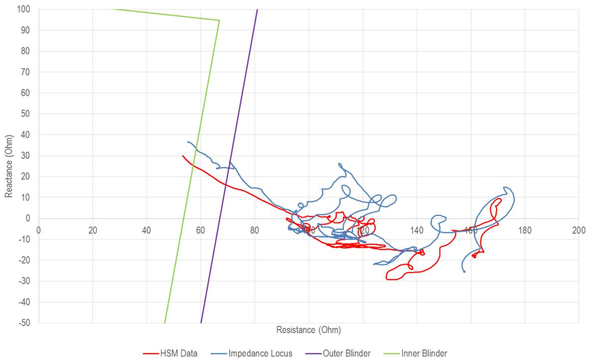
Figure 141 shows a good match between modelling and measured (HSM) values up to the point of system separation.
