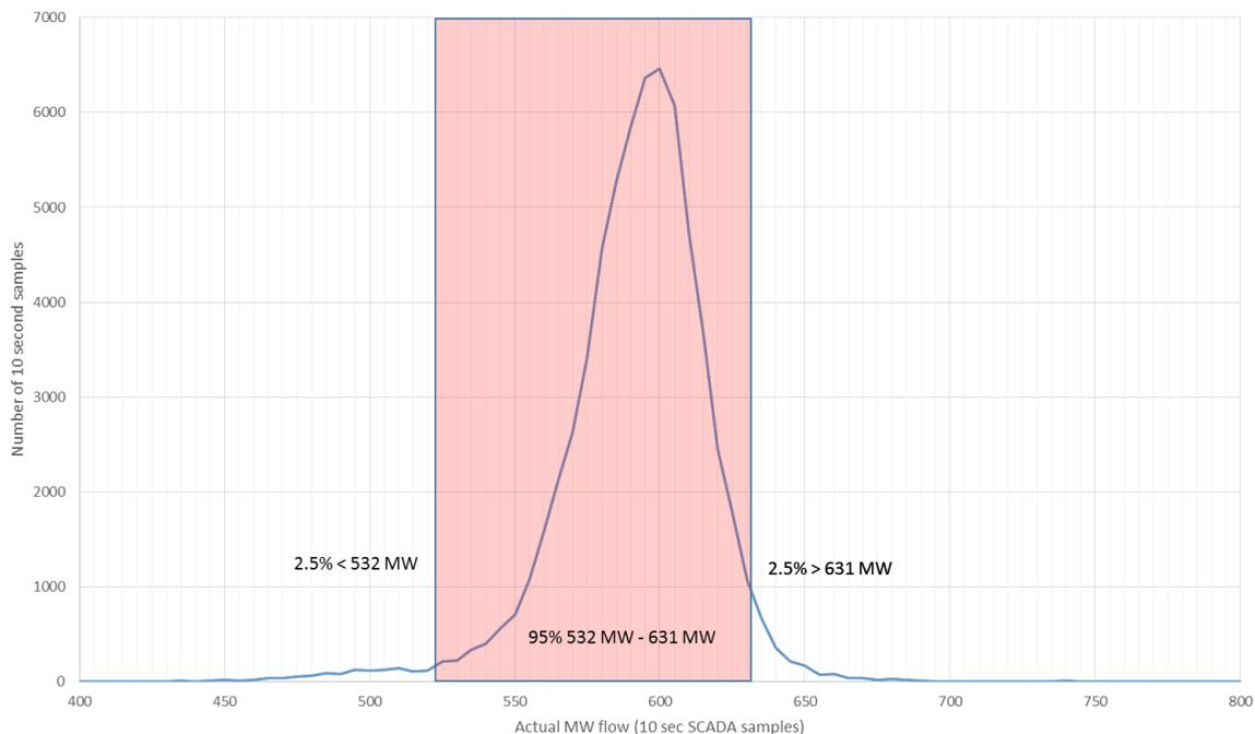
This analysis confirmed a drift of up to 30 MW in the actual flows, compared to the target flows.
