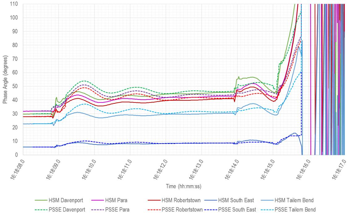
In Figure 137, differences can be observed between the modelled and measured (HSM) values of the Davenport frequency. This stems from the inability of the PSS/E and most other simulation tools to calculate the frequency under extreme operating conditions with abrupt changes in both voltage and frequency. This difference has no material impact on predicting whether loss of synchronism and islanding conditions will occur.
