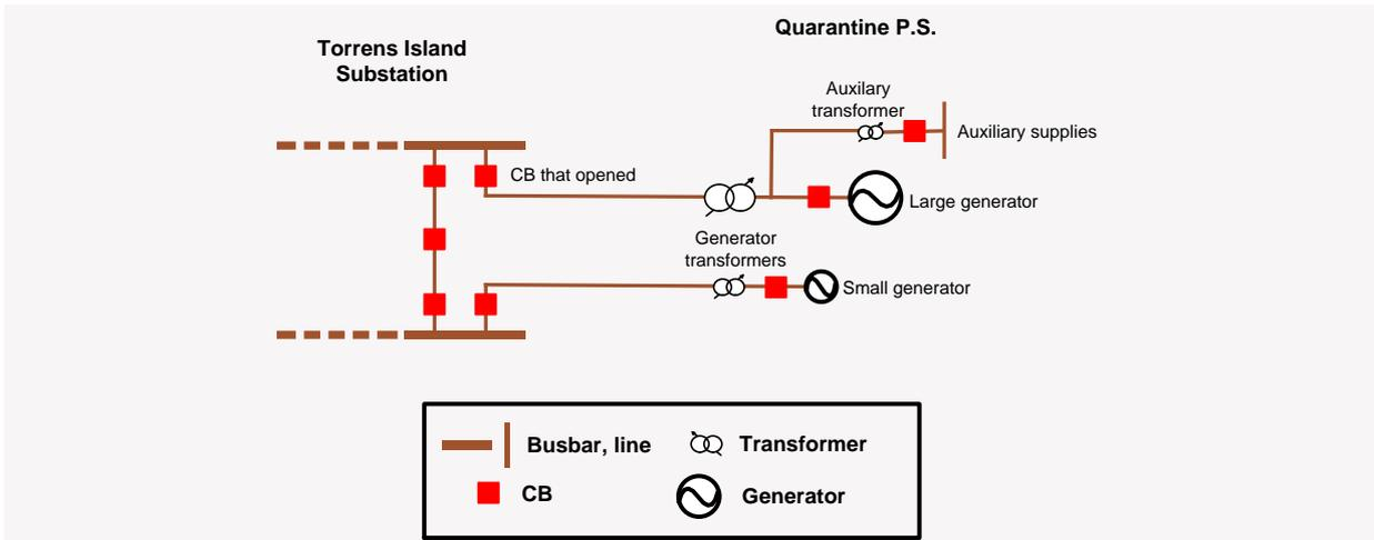
This problem had not been encountered during the test referred to in Appendix P or previous tests. Investigations by AEMO, ElectraNet, and Origin Energy have determined that a different switching sequence was used by ElectraNet on 28 September 2016 during the Black System than had been used for previous tests:
