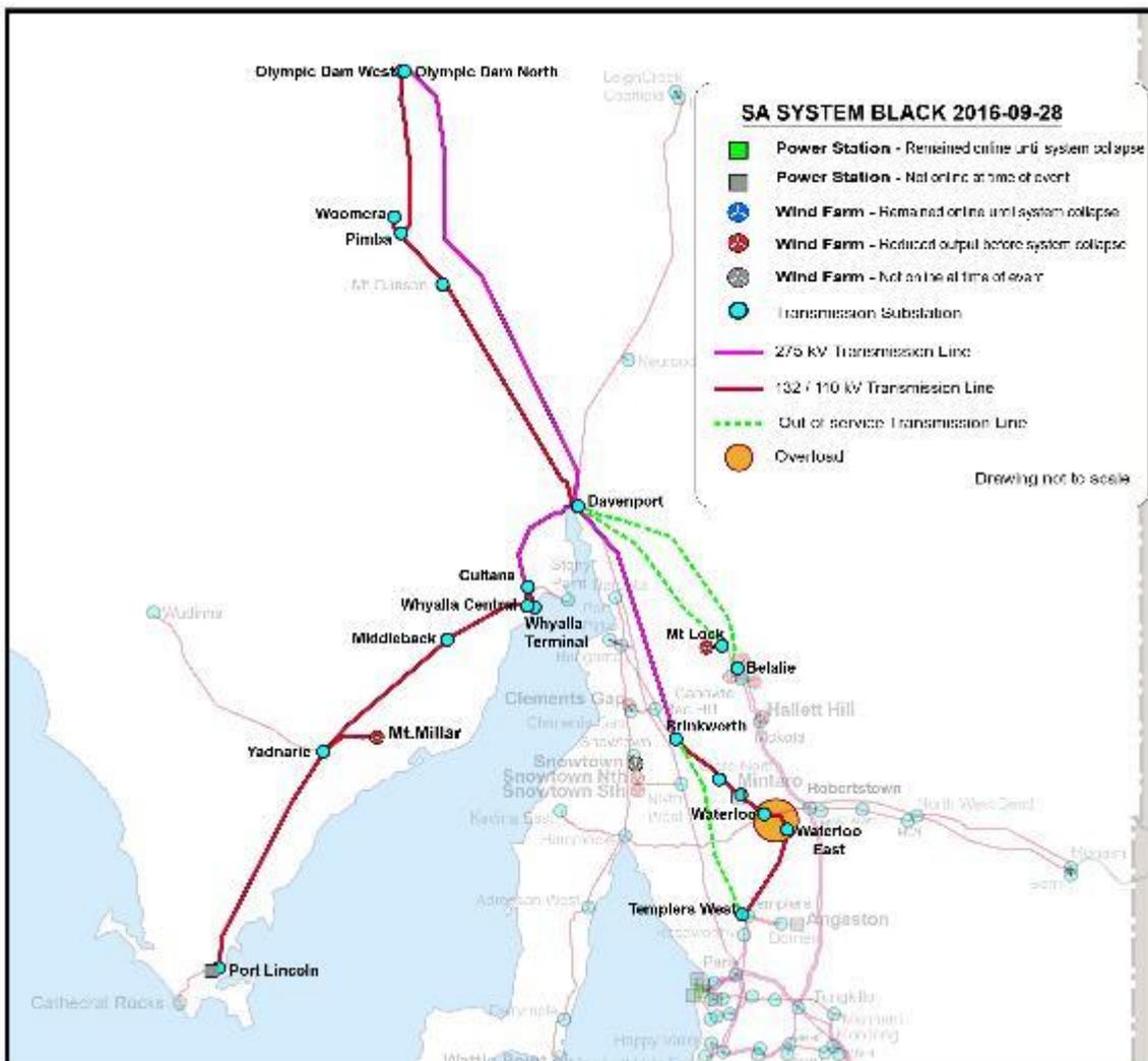
**Figure 79 Network capability with loss of four lines assuming no sustained power reduction by wind farms**
