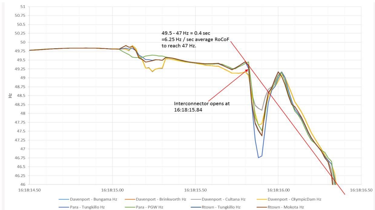
It is not clear whether these frequency measurements are a true reflection of power system frequency, or a transient frequency measurement or calculation issue, given the large and almost step changes in voltage phase angles in SA following separation (see Figure 13). These sudden angle changes, along with rapid changes in load due to possible operation of the UFLS scheme, may result in short-term inaccuracies in frequency measurements.
