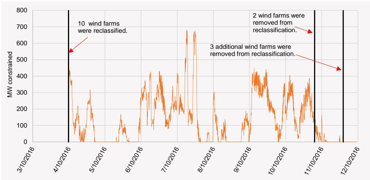
Due to AEMO’s inability to determine the cause of the Black System in the short term, it was not possible to ascertain the exact generation requirement to ensure AEMO was meeting its obligations to maintain power system security.<sup>88</sup> However, as it was suspected that inertia and system strength may have played a role in the system collapse, AEMO determined that the level of synchronous generation on-line should not fall below the level on-line prior to the Black System.
