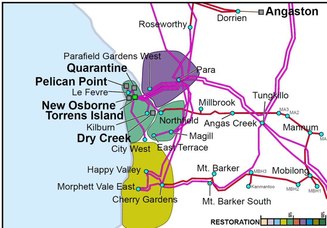
Figure 121 Percentage of load restored after 7 hours
