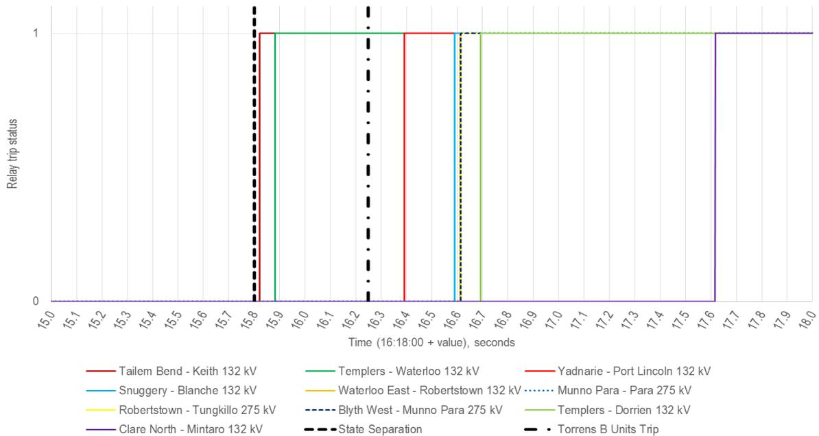
Close inspection of relay data indicates that all these relays operated on three-phase distance protection. However, as discussed in this report, all six voltage disturbances were unbalanced, for which operation of three-phase distance relays should be prevented.
