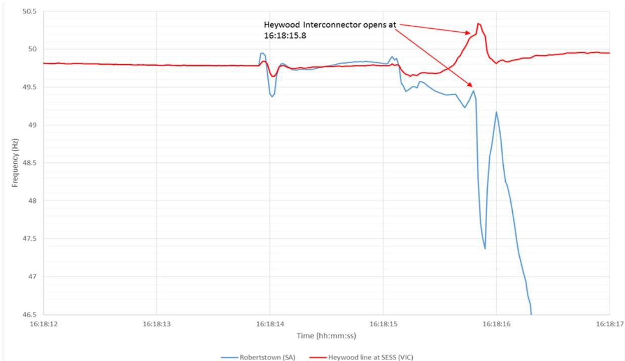
SA’s UFLS scheme is designed to quickly rebalance supply and demand, following any separation from Victoria which leaves SA short of supply.
