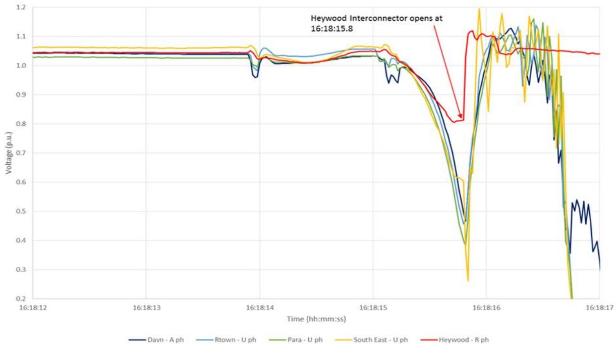
These six voltage disturbances resulted in depression of the generating systems’ connection point voltage for all on-line wind farms north of Adelaide. The impact of these voltage disturbances on fault ride-through response of all on-line wind farms in SA is discussed in Section 3.2.
