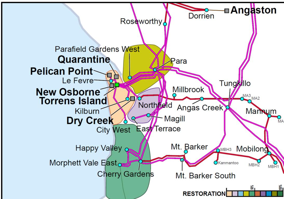
Figure 119 Percentage of load restored after 5 hours
