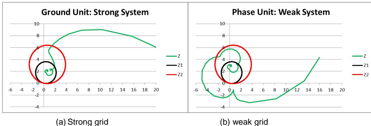
**Figure 186 Impact of system strength on fault direction seen by the distance relay**
