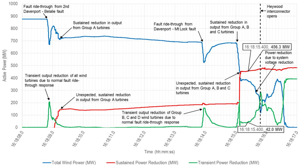
Figure 11 illustrates the power reduction of wind farms, based on the grouping in Table 9. It also highlights the following observations (noting the SA power system had experienced three voltage disturbances just prior to the time shown on Figure 11):
