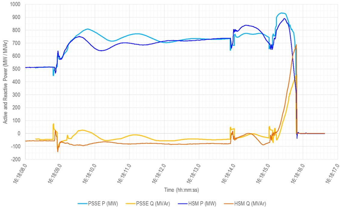
Figure 134 shows a good match between modelling and measured (HSM) values, with insignificant errors in simulating voltages at the time of system separation. This difference will have no impact on the ability to predict conditions resulting in loss of synchronism and whether a viable island can be formed.
