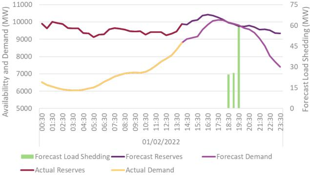
Figure 3 Forecast reserves position and operational demand at 1500hrs.
