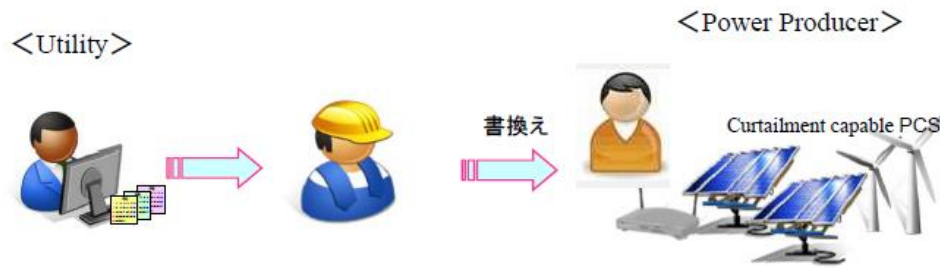
Figure 34: DER output control scheme without remote communications
